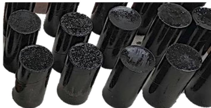
**Figure 4.** Preparation of cement asphalt mortar specimens.
