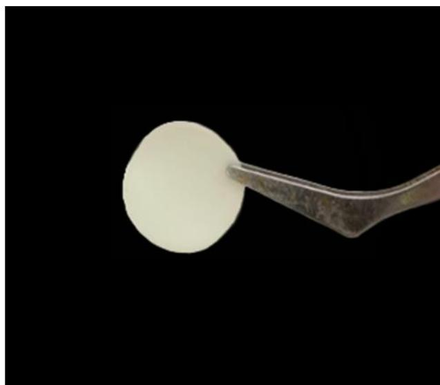
Figure 3. 3D printed plant-based GPE.
