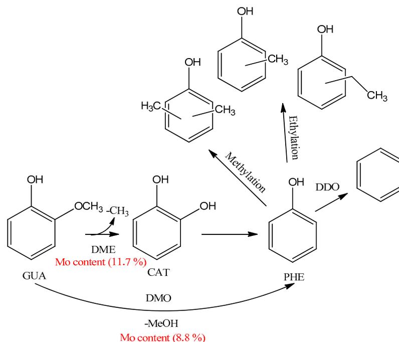
**Figure 5.** Supposed pathways of guaiacol conversion over the NiCuMo/SiO<sub>2</sub> catalysts based on [13,37,40,41].
