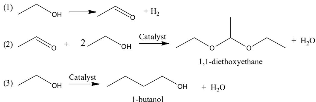
**Figure 1.** Formation of (1) acetal; (2) 1,1-diethoxyethane; and (3) 1-butanol during ethanol dehydrogenation.
