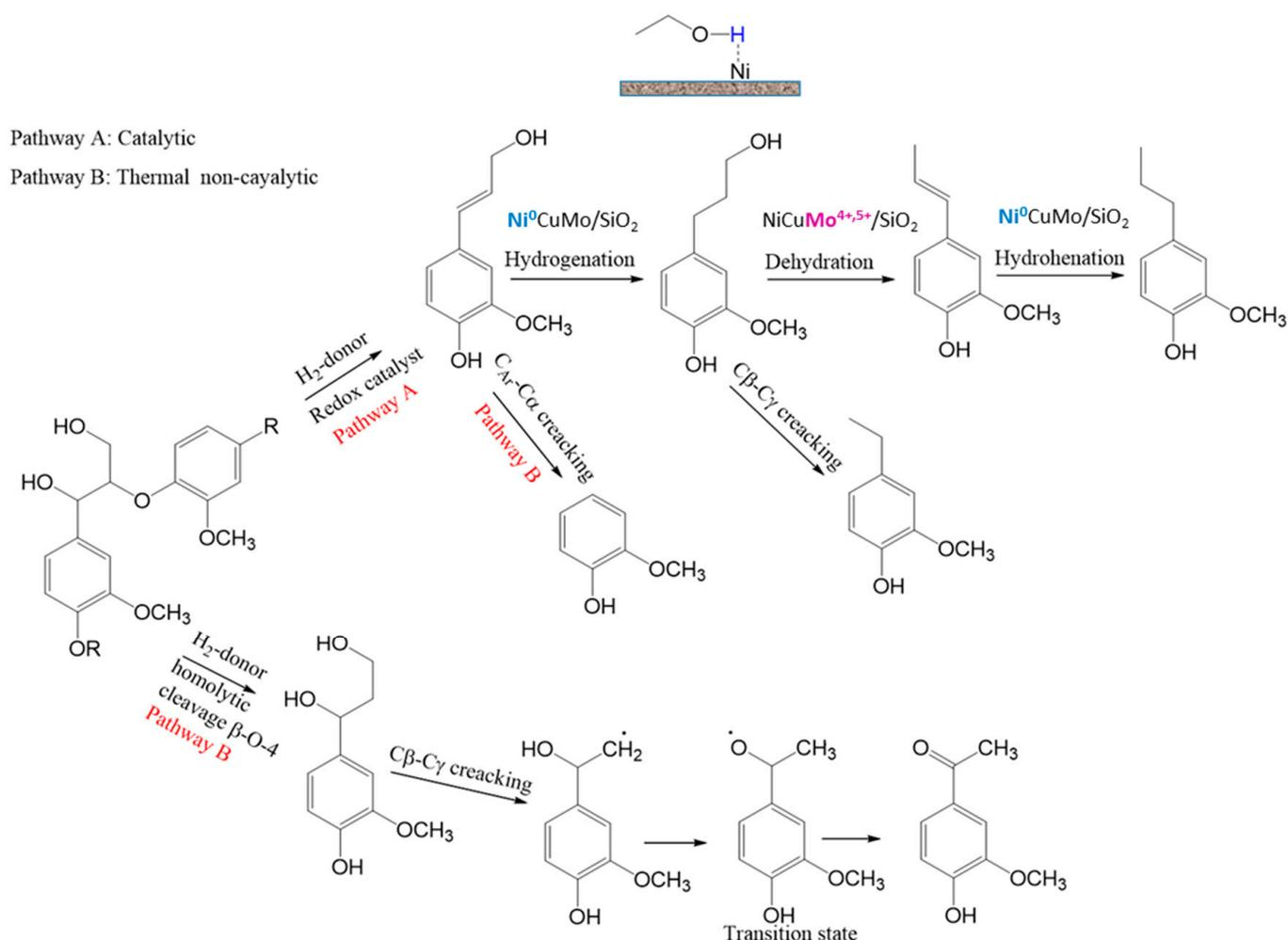
**Figure 4.** Catalytic (A) and non-catalytic (B) pathways of ethanol lignin depolymerization based on [33,35,37].
