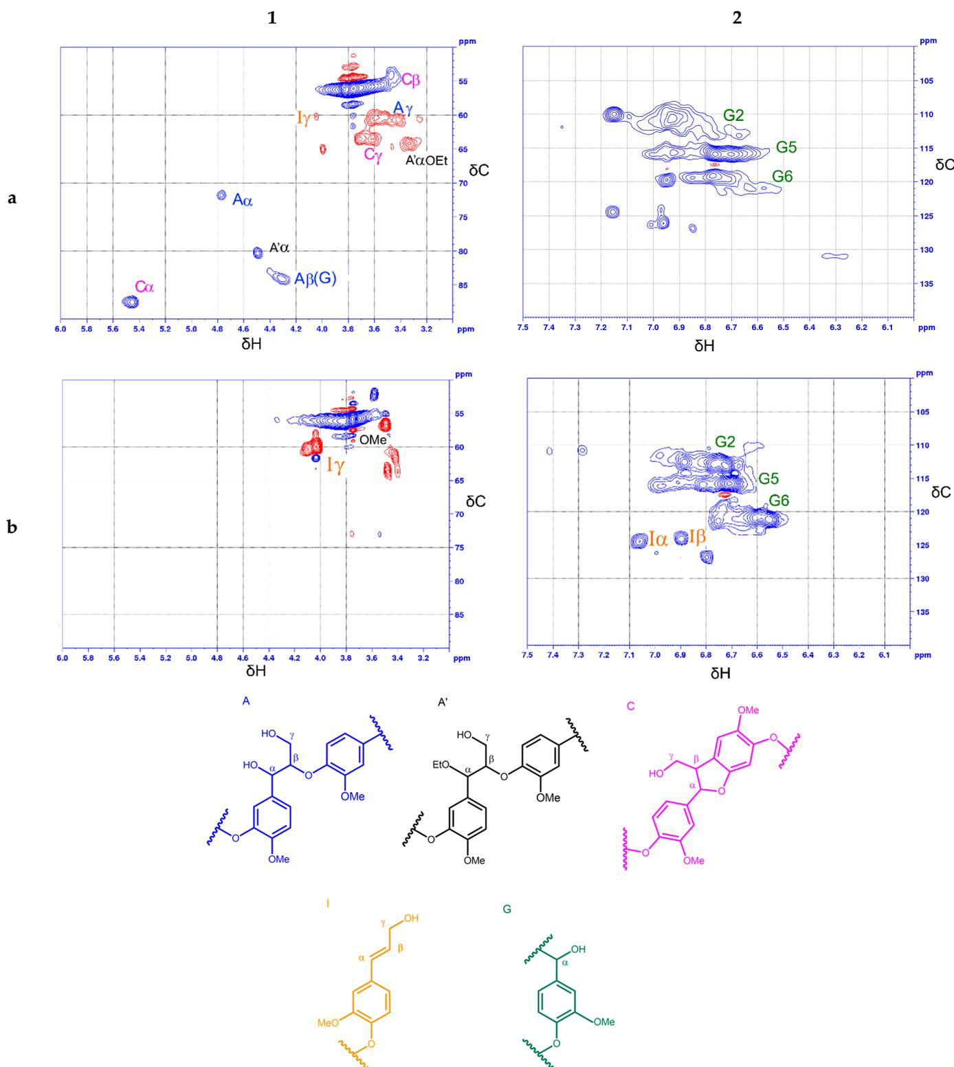
**Figure 2.** HSQC NMR spectra of (1) aliphatic oxygenated and (2) aromatic region: (a) pine ethanol lignin; (b) liquid products of its conversion over the NiCuMo/SiO<sub>2</sub>-1 catalyst in supercritical ethanol at 300 °C. Structural components: (A)  $\beta$ -aryl ether; (A') ethoxylated  $\beta$ -aryl ether; (C) phenylcoumarane; (I) coniferyl alcohol; (G) guaiacyl unit.
