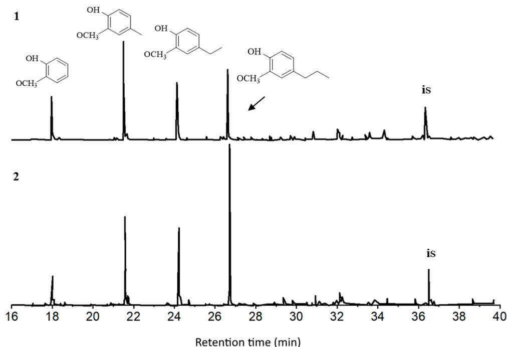
**Figure 3.** Chromatograms of monomer products of pine ethanol lignin conversion at 300 °C without catalyst (1) over the NiCuMo/SiO<sub>2</sub> catalyst (2). is—internal standard.
