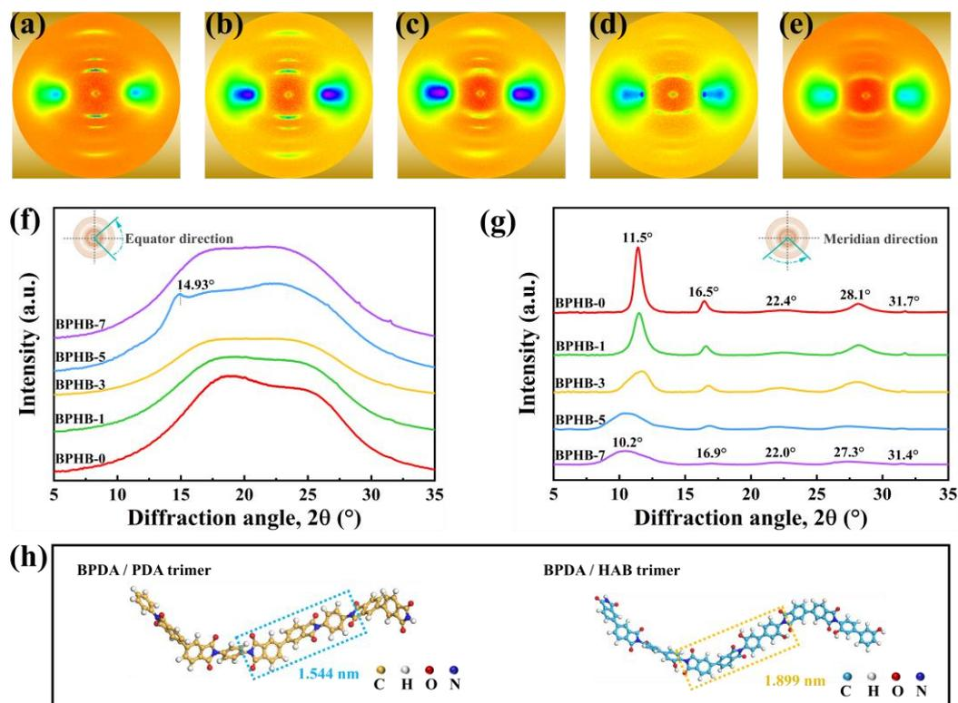
**Figure 2.** (a–e) 2D WAXD patterns for BPHB fibers with *p*-PDA/HAB/BIA molar ratios of 7/0/3, 6/1/3, 4/3/3, 2/5/3, and 0/7/3, respectively. (f) Equator and (g) meridian directions of the 1D WAXD profiles for the PI fibers with different *p*-PDA/HAB/BIA molar ratios. (h) Simulated conformations of BPDA/*p*-PDA and BPDA/HAB trimers, as well as the length of its repeat units, calculated by using the COMPASS force field of Materials Studio 8.0.
