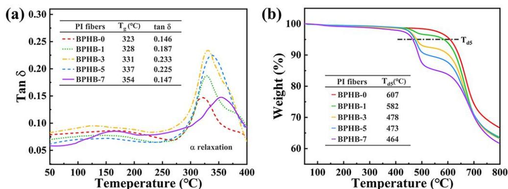
Figure 5. (a) DMA curves and (b) TGA curves of the PI fibers with different *p*-PDA/HAB/BIA molar ratios.
