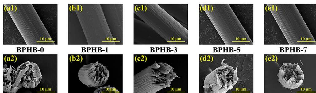
**Figure 3.** SEM images of the surface (a<sub>1</sub>–e<sub>1</sub>) and cross-section (a<sub>2</sub>–e<sub>2</sub>) of PI fibers.
