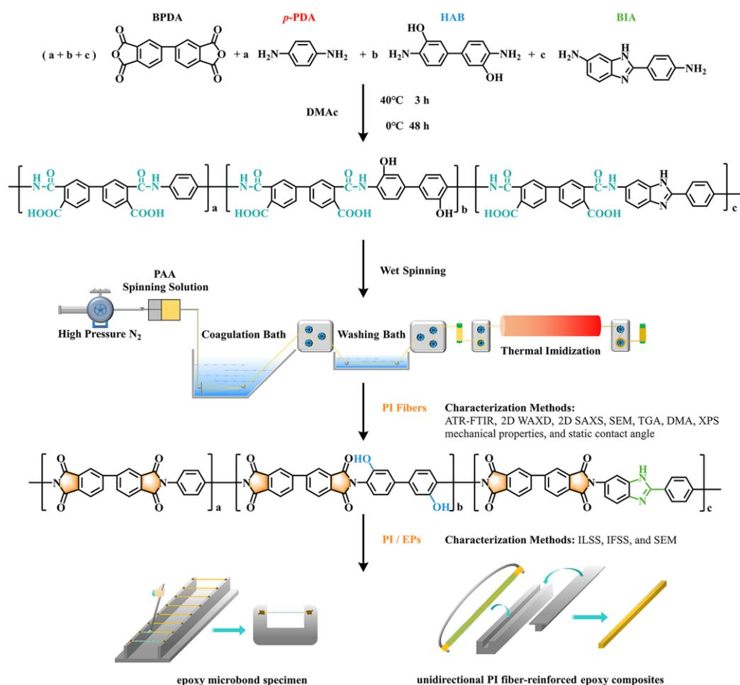
**Scheme 1.** Fabrication routes of PI fibers and PI/EPs.
