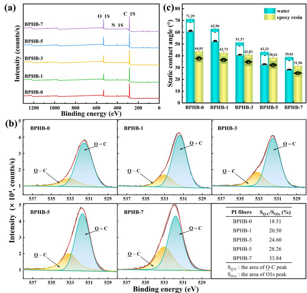
**Figure 6.** (a) XPS wide-scan spectra, and (b) curve-fitting O1s high-resolution XPS spectra for the BPHB fibers. (c) The static contact angle of water and epoxy resin for the prepared fibers.
