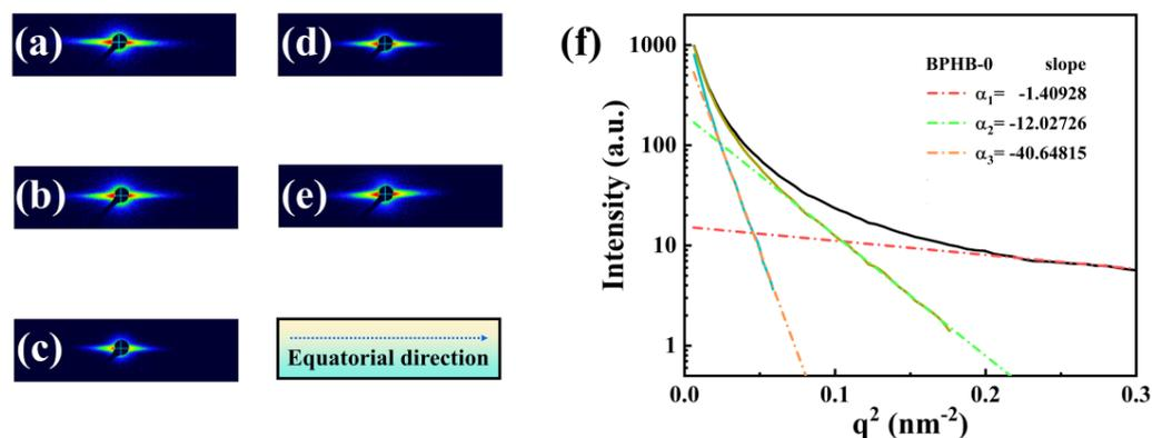
**Figure 4.** (a–e) 2D SAXS patterns for BPHB fibers with *p*-PDA/HAB/BIA molar ratios of 7/0/3, 6/1/3, 4/3/3, 2/5/3, and 0/7/3, respectively. (f) Guinier plot of the BPHB-0 fiber along the equator direction via Guinier functions and the Fankuchen successive tangent method.
