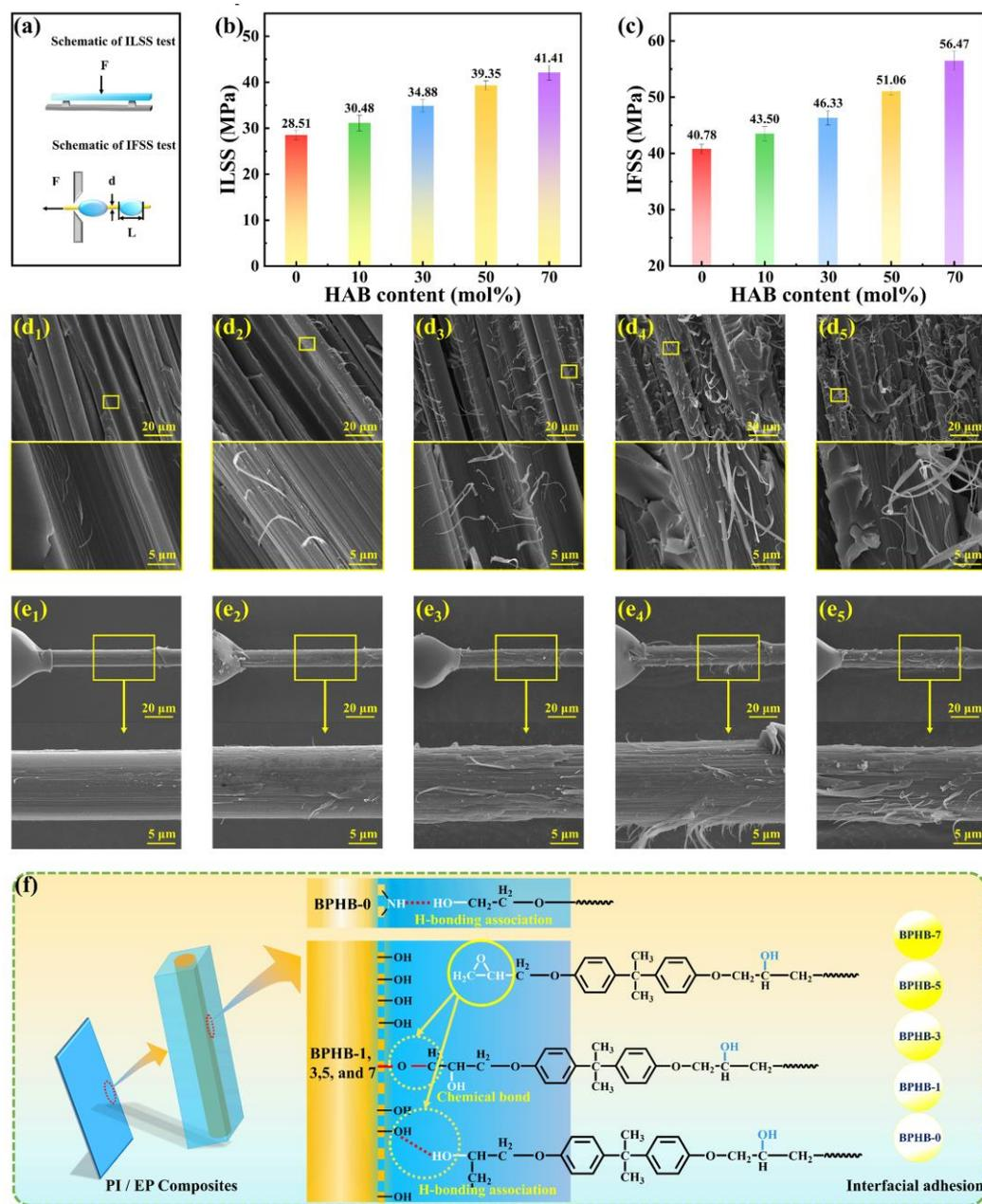
**Figure 7.** (a) Schematic of ILSS and IFSS test. (b) ILSS values and (c) IFSS values for the BPHB fibers. (d<sub>1</sub>–d<sub>5</sub>) Fracture images of the ILSS test, and (e<sub>1</sub>–e<sub>5</sub>) failure images of the IFSS test for the PI/EPs, in which the fibers have *p*-PDA/HAB/BIA molar ratios of 7/0/3, 6/1/3, 4/3/3, 2/5/3, and 0/7/3, respectively. (f) Interfacial interaction mechanism of the unidirectional PI/EPs.
