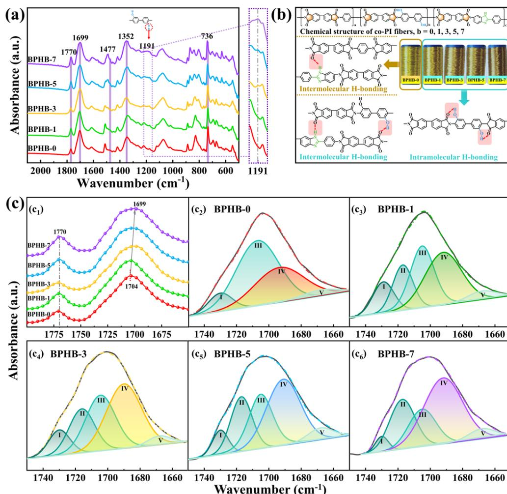
**Figure 1.** (a) ATR-FTIR spectra of the PI fibers with the different *p*-PDA/HAB/BIA molar ratios. (b) Intra-/intermolecular H-bonding interactions in BPHB fibers. (c<sub>1</sub>) Magnified ATR-FTIR spectra of PI fibers at the wavenumber range of  $1800\text{--}1650\text{ cm}^{-1}$ ; (c<sub>2</sub>–c<sub>6</sub>) curve-fitting ATR-FTIR spectra in the wavenumber range from  $1650\text{ cm}^{-1}$  to  $1750\text{ cm}^{-1}$ .
