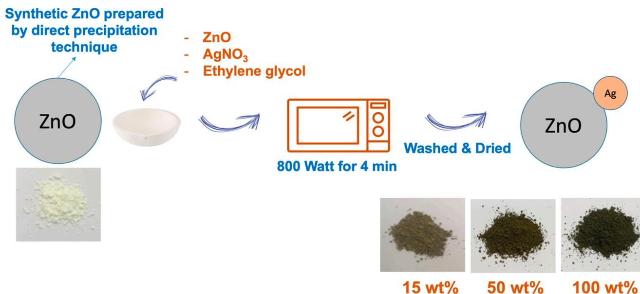
**Figure 1.** Schematic illustration regarding the steps for synthesis of Ag-doped ZnO.
