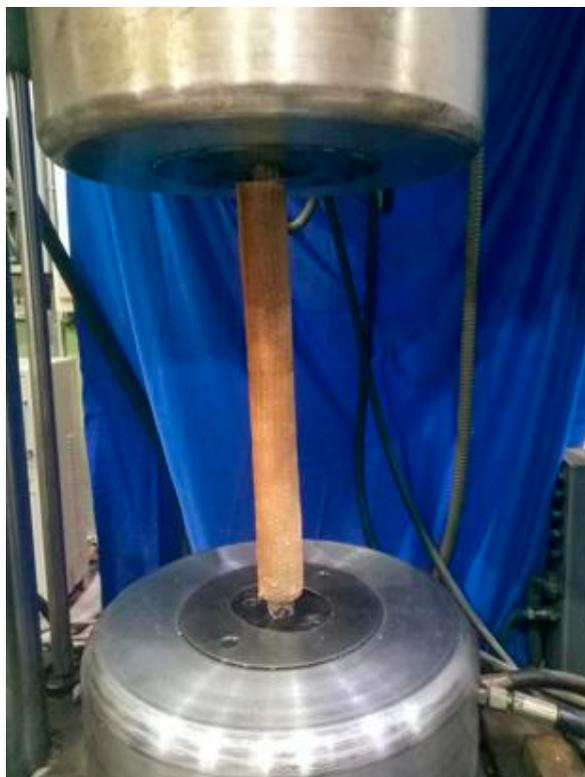
**(a)** Scene diagram.
