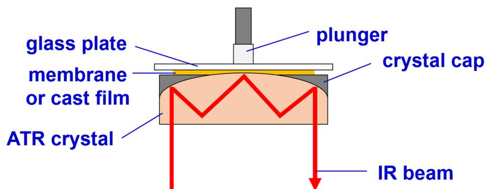
**Figure 3.** The setup for performing FTIR/ATR analysis at the surface of a membrane or a cast film.
