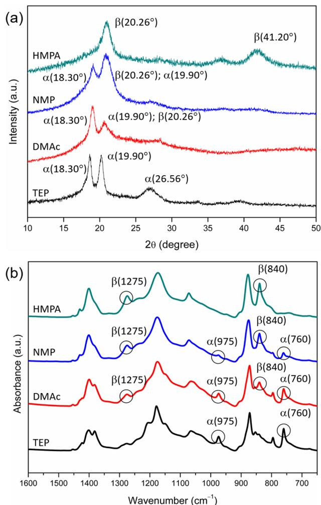
**Figure 5.** XRD (a) and FTIR/ATR (b) spectra of the surfaces of PVDF membranes prepared with nonsolvent-induced phase separation, with HMPA, NMP, DMAc or TEP used as the solvent to dissolve PVDF.
