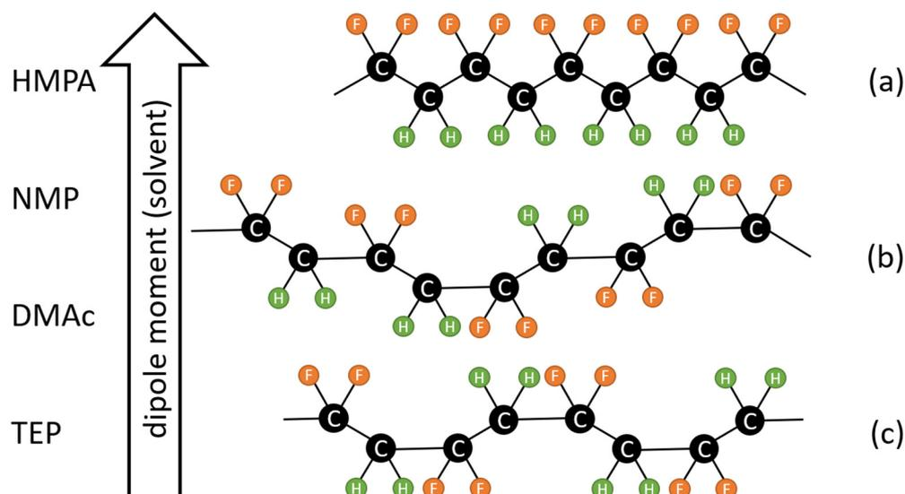
**Figure 1.** Relationship between PVDF chain conformation and the dipole moment of solvent. PVDF is inclined to form a more polar solution state conformation as it dissolves in a solvent with a higher dipole moment. (a) All tans (TTTT); (b) TTTG; and (c) TGTG'.
