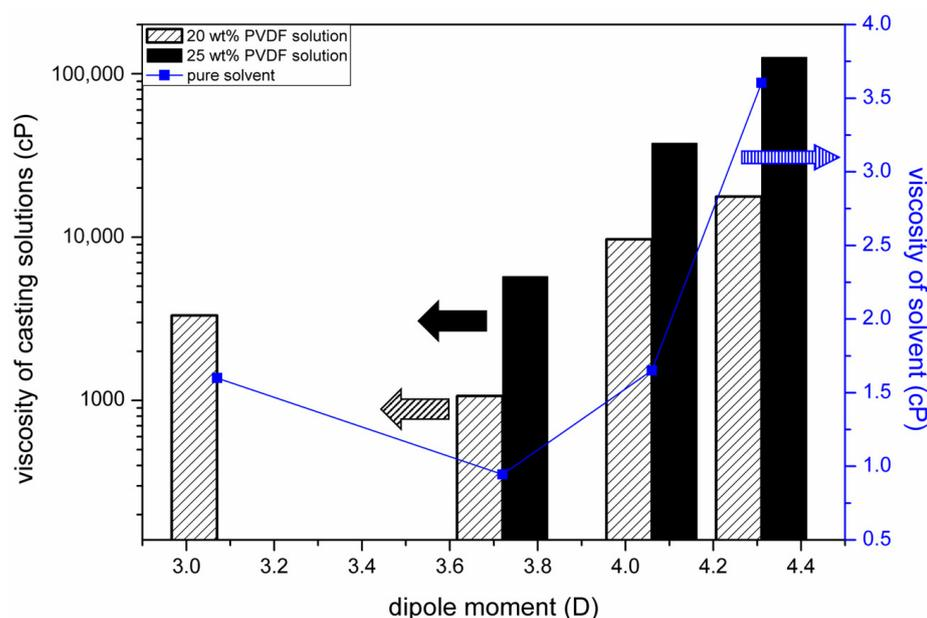
**Figure 11.** Dependence of the viscosities of solvents and casting solutions on solvent dipole moments.
