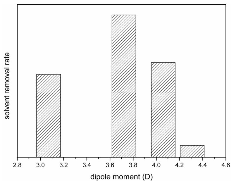
**Figure 10.** Schematic presentation of the dependence of the solvent removal rate in coagulation bath on its dipole moment.
