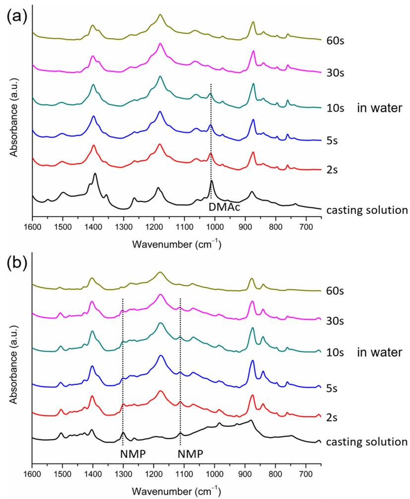
**Figure 9.** FTIR/ATR spectra of the surfaces of PVDF cast films at different times after immersion in water, with DMAC (a) or NMP (b) as the solvent.
