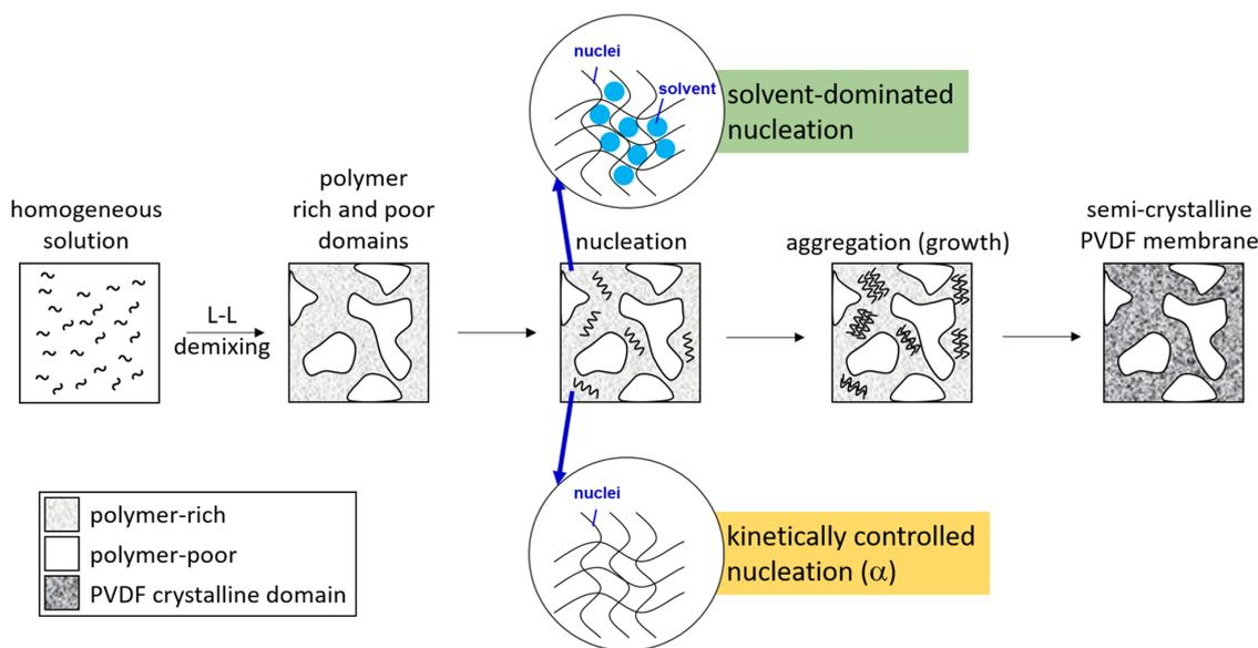
**Figure 7.** Schematic presentation of the formation mechanism of PVDF membranes.
