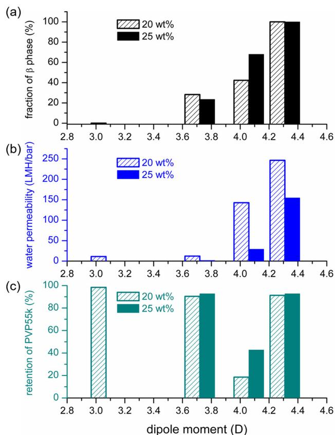
**Figure 8.** Dependence of the fractions of  $\beta$ -crystalline phase (a), water permeabilities (b) and retention of PVP (c) of PVDF membranes on the dipole moments of the solvents used to dissolve PVDF.
