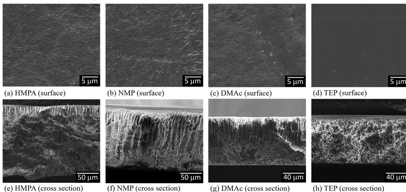
**Figure 4.** SEM images of the surfaces and cross-sections of PVDF membranes prepared with nonsolvent-induced phase separation, with HMPA, NMP, DMAc or TEP used as the solvent to dissolve PVDF.
