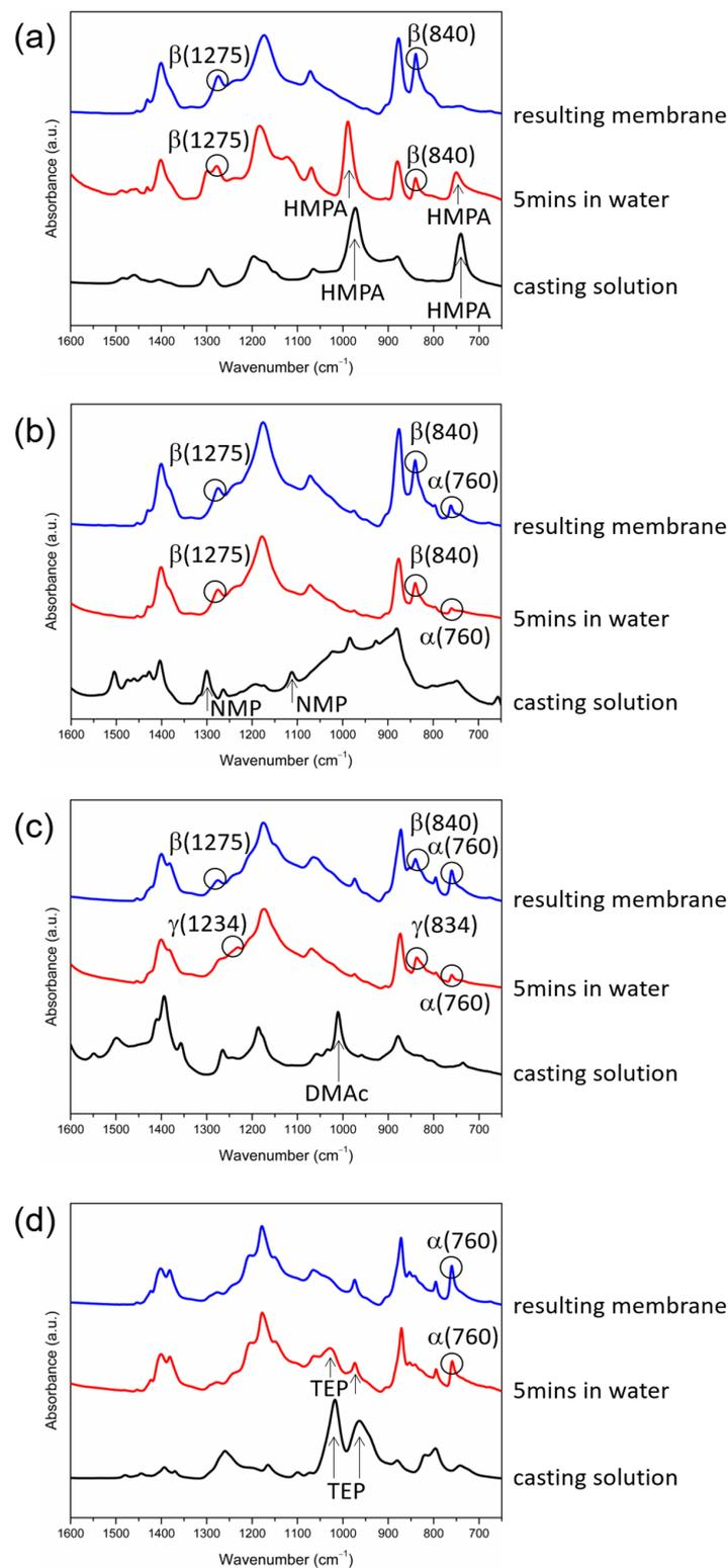
**Figure 6.** FTIR/ATR spectra of the surfaces of PVDF cast films at three time points during membrane formation (immediately after the solution casting, after 5 min in water, and after the membranes were formed) with HMPA (a), NMP (b), DMAc (c) or TEP (d) as the solvent.
