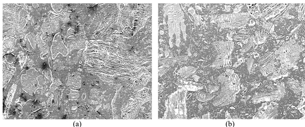
**Figure 3.** Scanning electron micrographs of the surfaces of PP/OPTP composites (70% pulp/26% PP/4% Exxelor PO 1020) produced with a pressing pressure of 50 tonnes and with (a) unheated and (b) 80 °C mould temperatures at 100× magnification.
