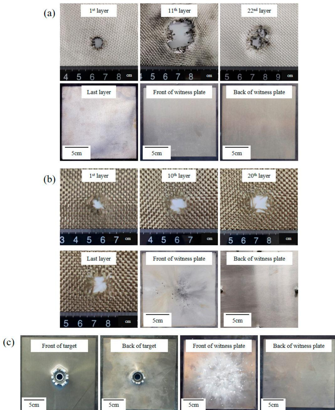
**Figure 4.** Results of HVI experiment for (a) UHMWPE fabric (S3, 4.250 km/s); (b) Basalt fabric (S1, 4.190 km/s); (c) Al plate (S2, 4.266 km/s).
