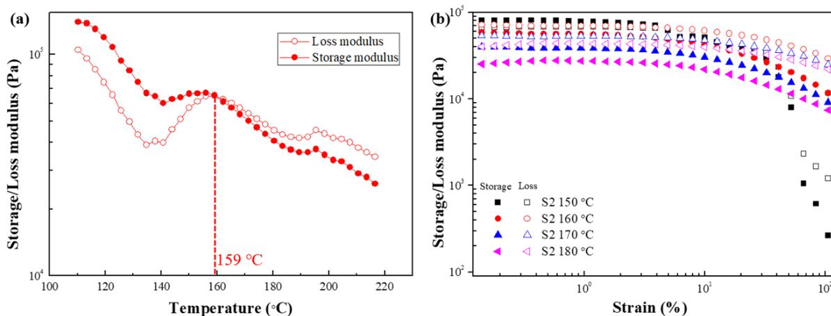
**Figure 8.** Storage (closed symbols) and loss (open symbols) modulus of (a) temperature sweep test and (b) strain amplitude sweep test for S2.
