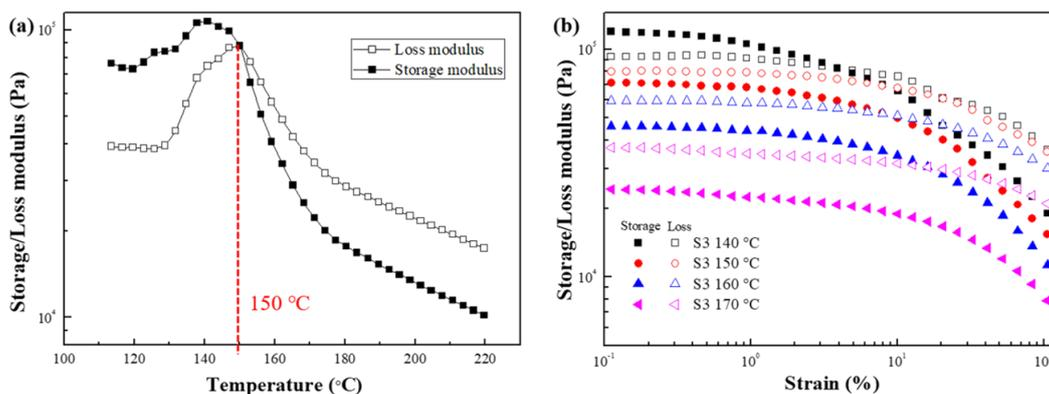
Figure 12. Storage (closed symbols) and loss (open symbols) modulus of (a) temperature sweep test and (b) strain amplitude sweep test for S3.
