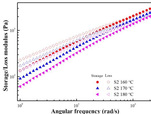
Figure 11. Frequency-dependent storage modulus (closed symbols) and loss modulus (open symbols) of S2 at various temperatures.
