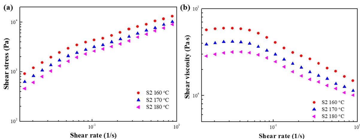
**Figure 9.** (a) Shear stress and (b) shear viscosity as a function of shear rate for S2 at various temperatures.
