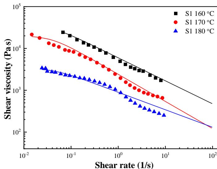
**Figure 6.** Shear viscosity as a function of the shear rate for S1 at various temperatures. The solid lines were fitted using the Carreau model.
