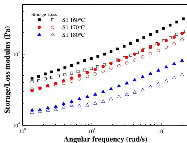
**Figure 7.** Frequency-dependent storage modulus (closed symbols) and loss modulus (open symbols) of S1 at various temperatures.
