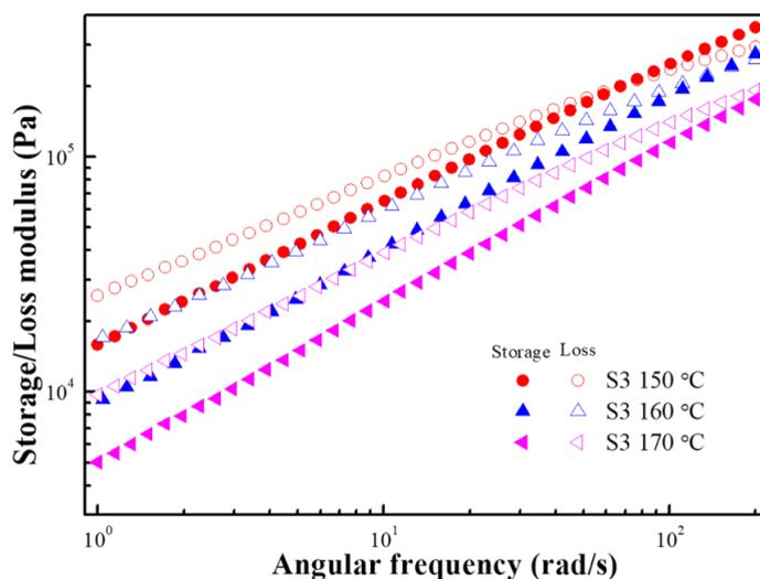
**Figure 15.** Frequency-dependent storage modulus (closed symbols) and loss modulus (open symbols) of S3 at various temperatures.
