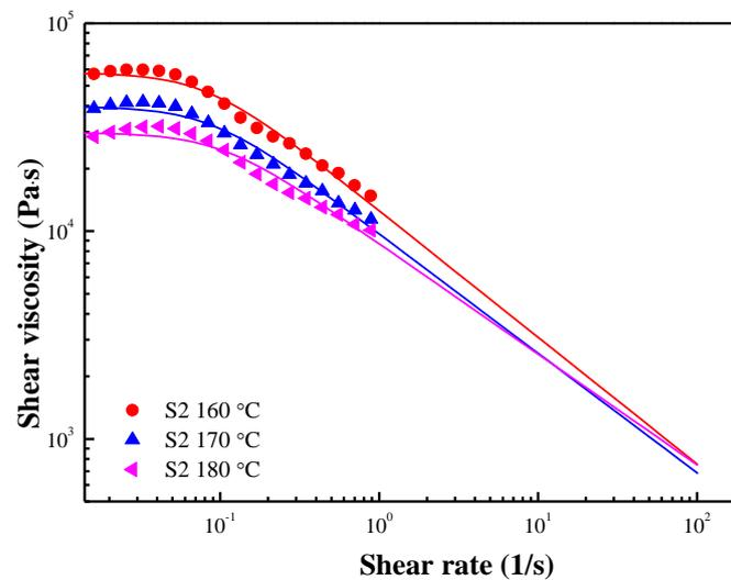
**Figure 10.** Shear viscosity as a function of shear rate for S2 at various temperatures. The solid lines were fitted by the Carreau model.
