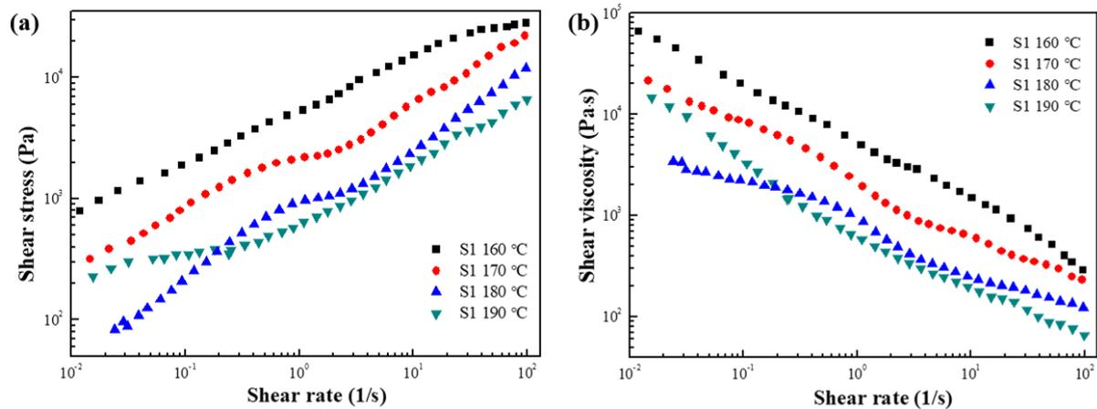
**Figure 5.** (a) Shear stress and (b) shear viscosity as a function of shear rate for S1 at various temperatures.
