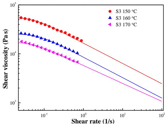
Figure 14. Shear viscosity as a function of the shear rate for S3 at various temperatures. The solid lines are fitted by the Carreau model.
