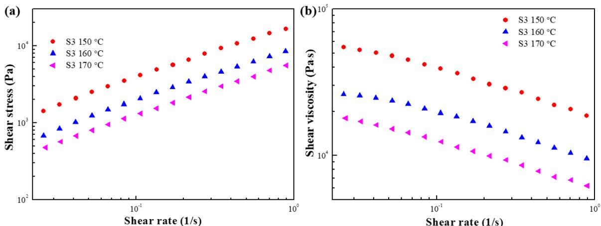
Figure 13. (a) Shear stress and (b) shear viscosity as a function of the shear rate for S3 at various temperatures.
