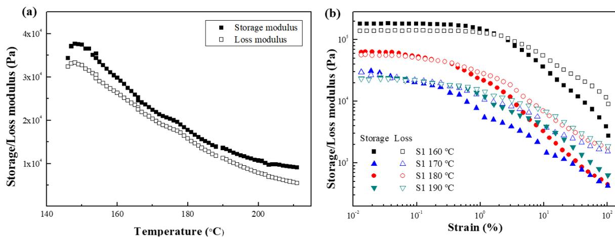
Figure 4. Storage (closed symbols) and loss (open symbols) modulus of (a) temperature sweep test and (b) strain amplitude sweep test for S1 at various temperatures.
