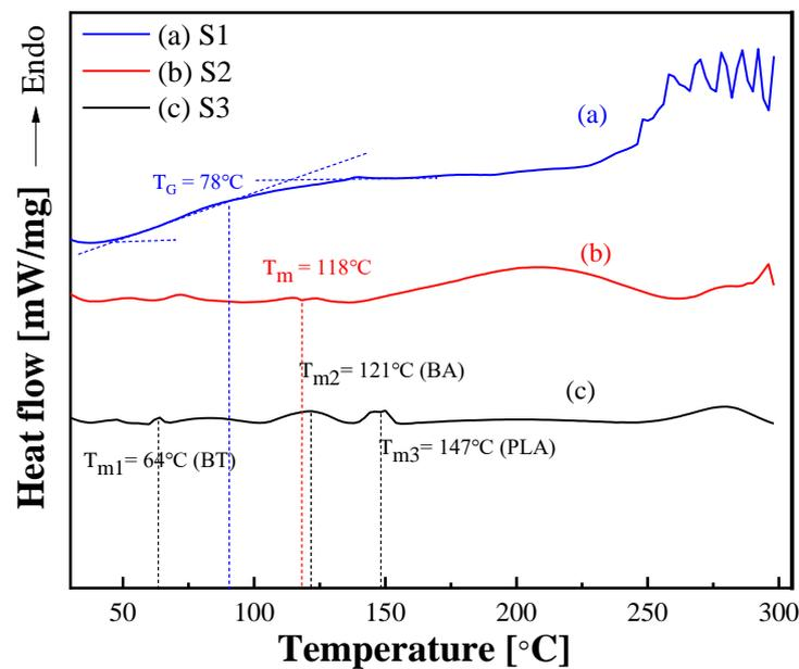
Figure 3. DSC curves of (a) S1, (b) S2, and (c) S3.
