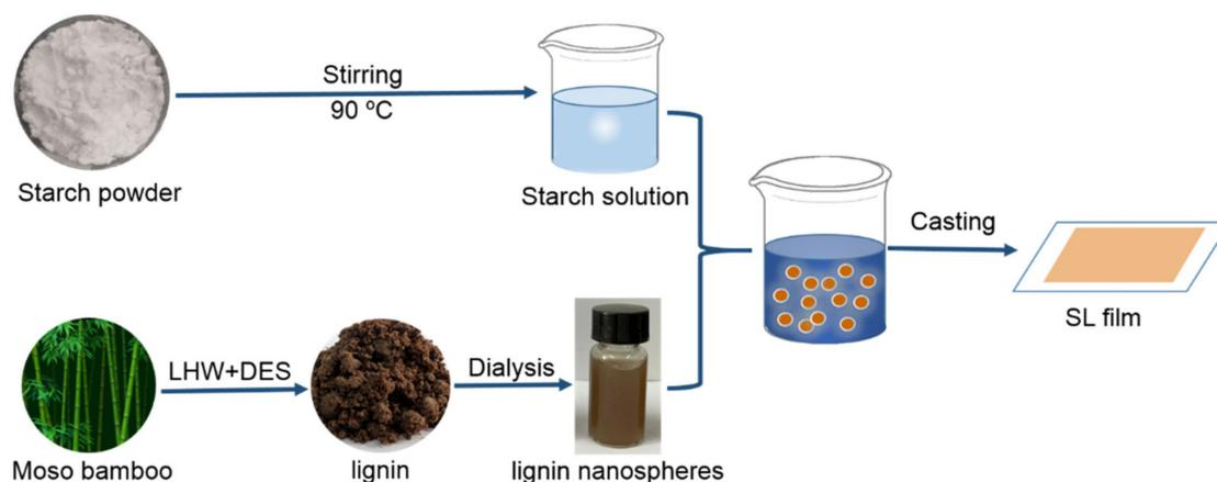
**Scheme 1.** Schematic illustrating of fabrication process of Starch/LNPs composite film.
