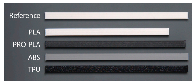
Figure 7. Effect of thermal activation on the longitudinal shrinkage of 3D-printed samples compared to a reference sample before thermal activation.
