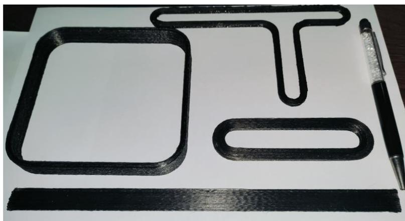
**Figure 19.** High-throughput multifilament additive manufactured parts of CCFRP.
