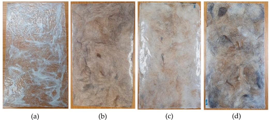
**Figure 5.** Composite laminates produced—(a) Fiberglass composite; (b) Dog wool fibers without treatment composite; (c) Dog wool fibers with PVA treatment composite; (d) Dog wool fibers with NaOH treatment composite.
