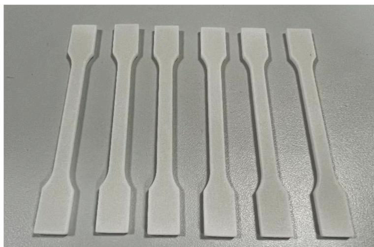
**Figure 1.** Standard samples with a 2 mm thickness.
