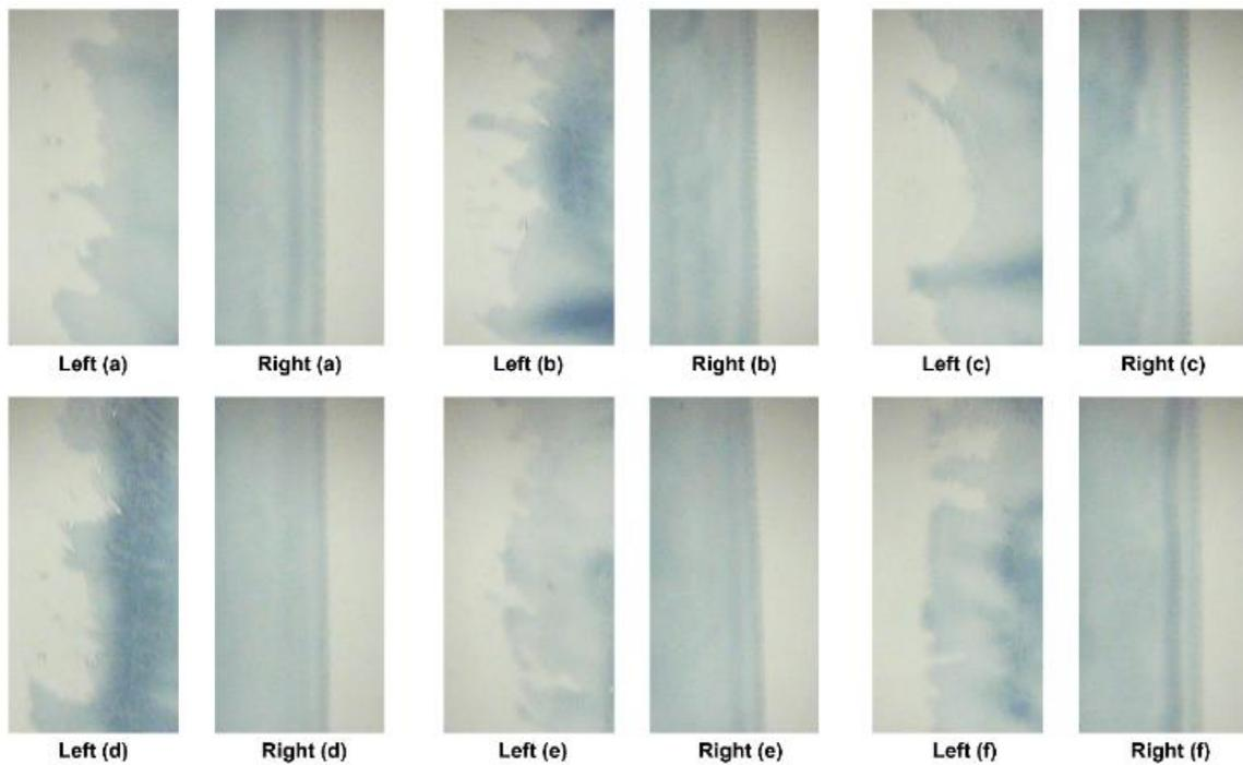
**Figure 9.** Vision images captured after drying: edge defects (**left**) and normal conditions (**right**). (a–f) Defect and Normal conditions for after dryer.
