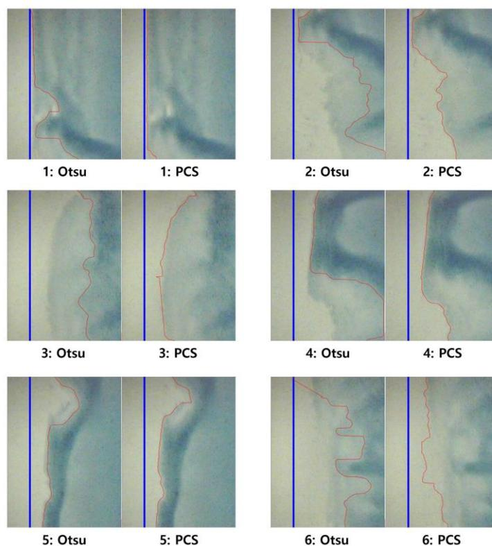
**Figure 12.** Comparison of edge detection results: Otsu’s method vs. PCS.
