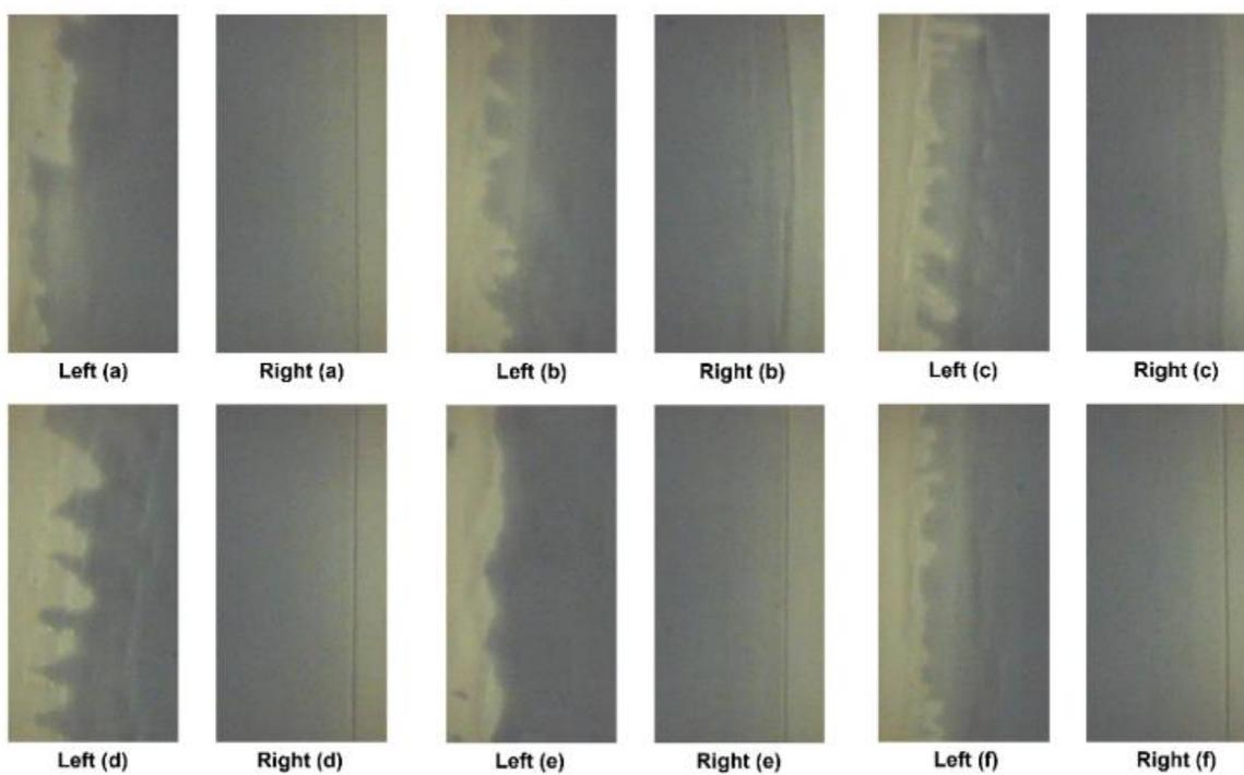
**Figure 10.** Vision images captured before drying: edge defects (**left**) and normal conditions (**right**). (a–f) Defect and Normal conditions for before dryer.
