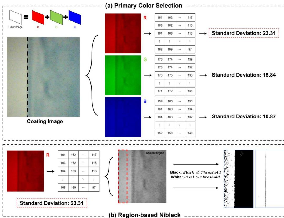
Figure 4. Schematic of the PCS and RN methods.
