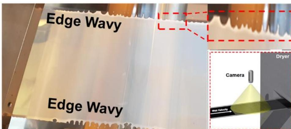
Figure 2. Examples of edge defects in an R2R manufacturing system.
