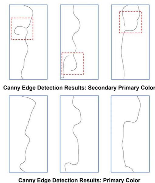
Figure 13. Comparison of Canny edge detection result based on primary and secondary color.
