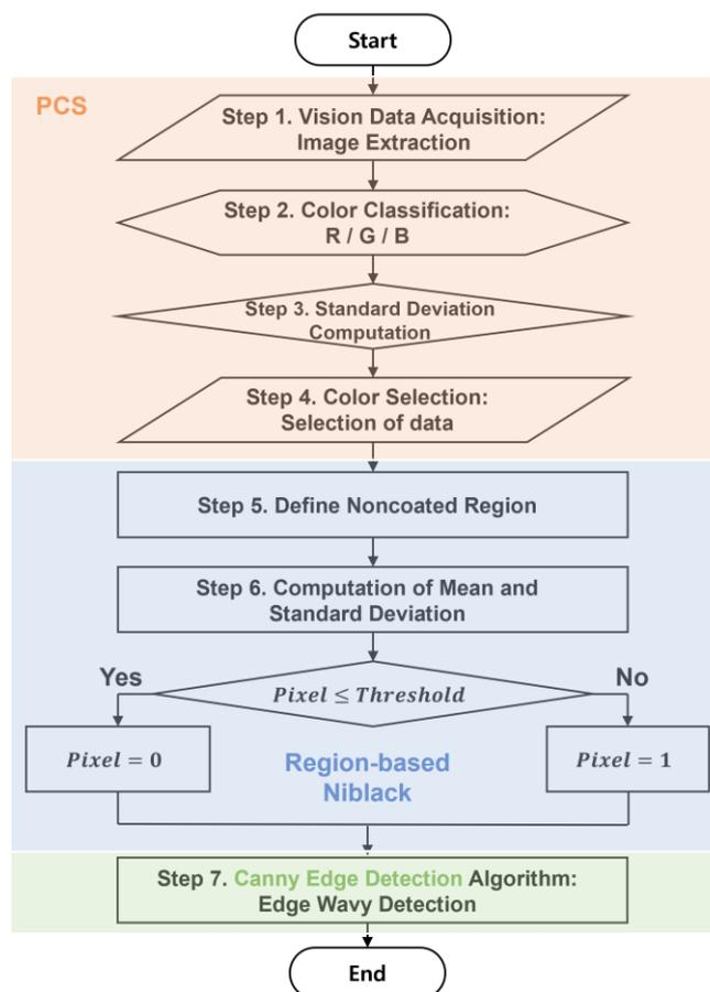
**Detection of Edge Wavy Defect with PCS Method**
