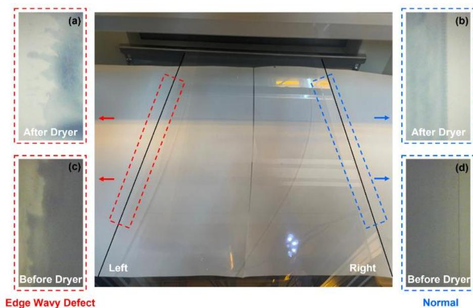
Figure 8. Comparison of the coating structural quality of coatings with and without edge defects. (a) Edge wave defect after dryer. (b) Edge wave defect before dryer. (c) Normal condition after dryer. (d) Normal condition before dryer.
