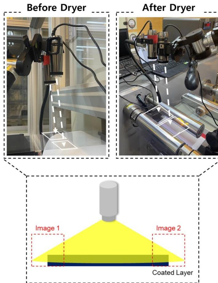
Figure 7. Vision camera setup of the R2R slot-die coater for edge detection.
