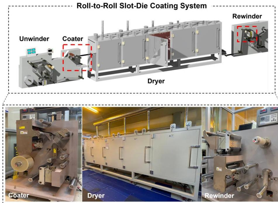
Figure 1. Roll-to-roll (R2R) slot-die coating system.
