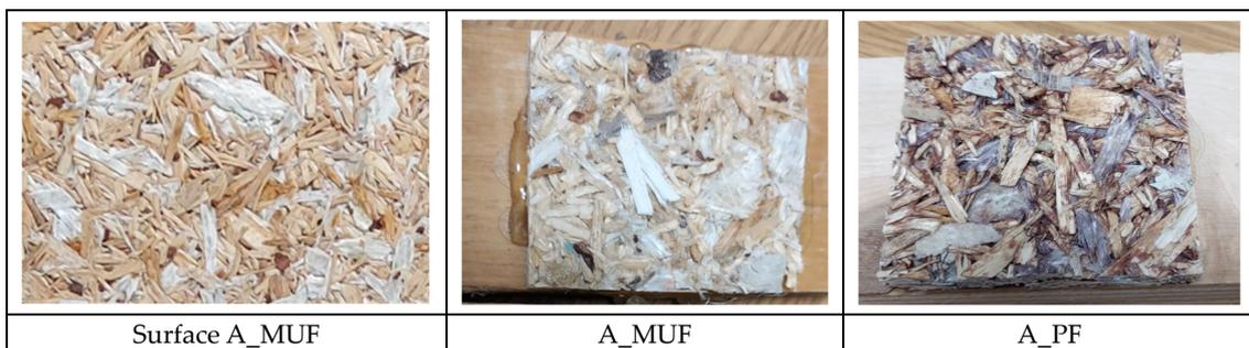
**Figure 6.** Appearance of the boards after the tensile strength test perpendicular to the surfaces.
