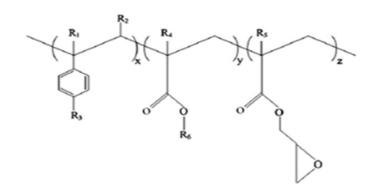
Figure 2. General structure of reactive oligomers (chain extenders).
