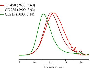
**Figure 5.** GPC traces of stearic acid grafted epoxy functional reactive oligomers with low, medium and high functionality before and after reaction.
