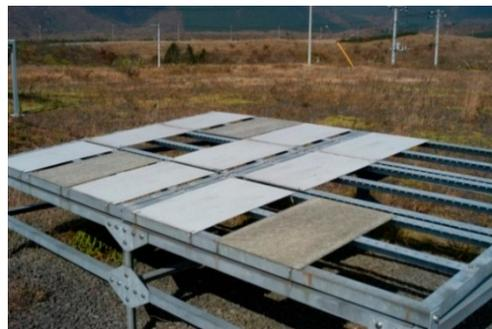
Figure 3. Specimens placed on exposure racks facing south on a 5° slope.
