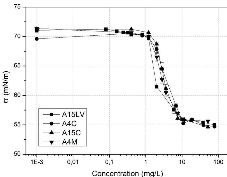
**Figure 11.** Influence of the molecular weight on the tension-active properties ( $\sigma$  in mN/m) of MC with different molecular weights as a function of polymer concentration at 20 °C. The lines are added to guide the eye [24].
