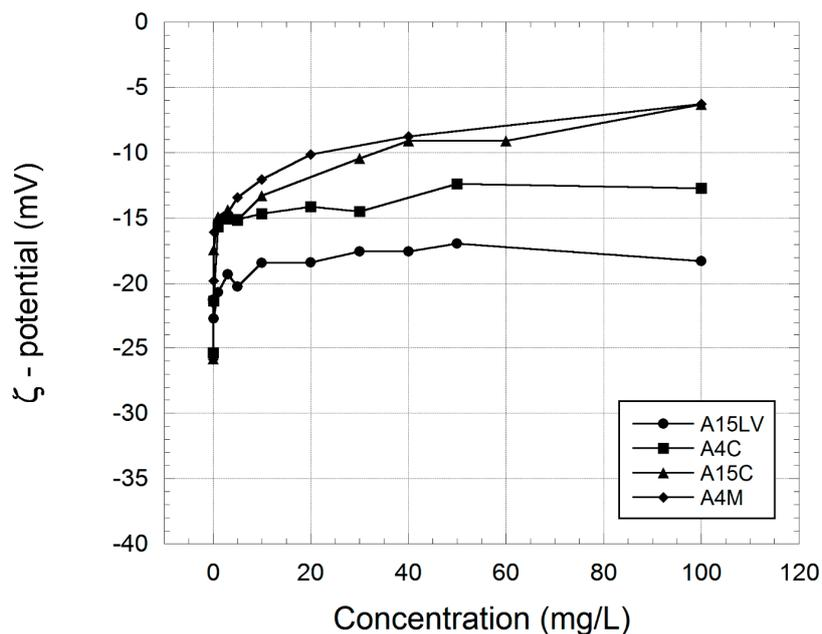
**Figure 12.**  $\zeta$ -Potential (expressed in mV) of silica particles with an average 0.5- $\mu\text{m}$  diameter dispersed in water at 20 °C in the presence of increased amounts of methylcelluloses with different molecular weights. The lines are added to guide the eye [24].
