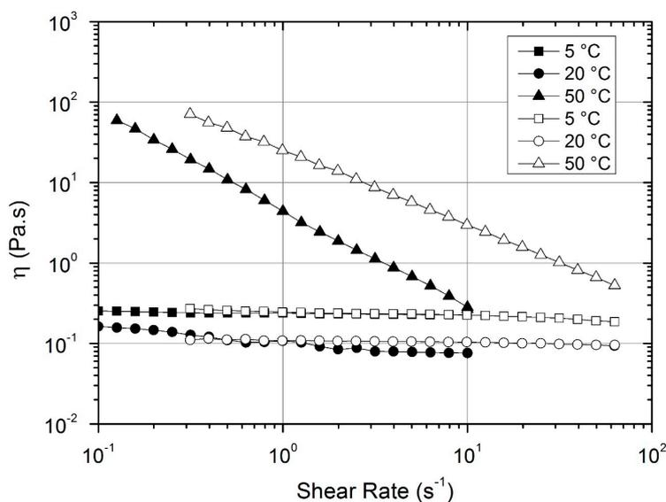
**Figure 5.** Viscosity as a function of the shear rate for methylcellulose A15C at 10 g/L. Open symbols are given for Cox–Merz transformation of dynamic measurements, filled symbols are for flow measurements. The lines are added to guide the eye.
