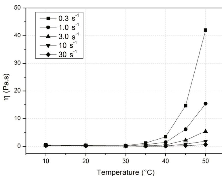
**Figure 6.** Influence of temperature on the viscosity of methylcellulose solution at different shear rates. Viscosities of a 10 g/L solution of A4M obtained using Cox–Merz transformation of dynamic measurements in the linear viscoelastic region. The lines are added to guide the eye [24].
