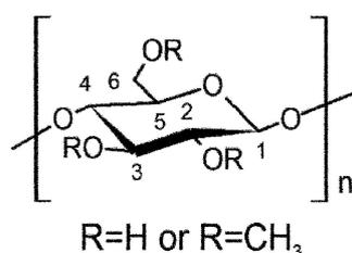
**Figure 1.** Repeating unit of methylcellulose:  $-\text{OH}$  or  $-\text{OCH}_3$  at positions 2, 3 and 6 of the anhydro-D-glucose.
