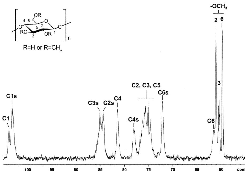
**Figure 2.**  $^{13}\text{C}$ -NMR spectrum of methylcellulose A4C (30 g/L in DMSO- $d_6$  at 80 °C). C<sub>x</sub> and C<sub>xs</sub> correspond to the signals of carbon *x* unsubstituted and substituted, respectively. Reproduced with permission from Taylor & Francis Group, 2015 [20].
