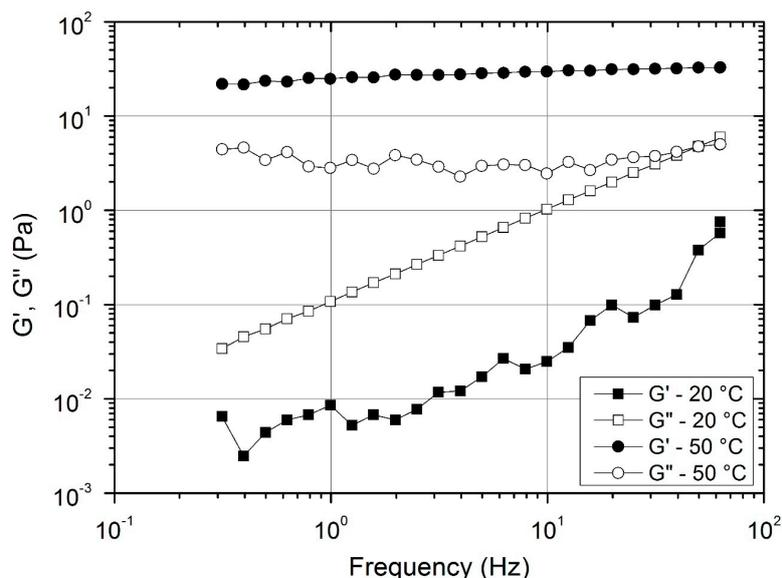
**Figure 7.** Dynamic behavior of methylcellulose A15C at 10 g/L in aqueous solution.  $G'$  filled symbols (at 20 °C, the values remain difficult to determine due to their magnitude around  $10^{-2}$  Pa),  $G''$  open symbols. The lines are added to guide the eye.
