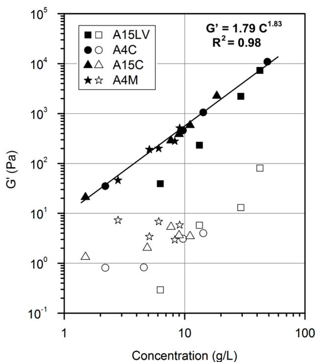
**Figure 10.** Storage moduli  $G'$  as a function of the polymer concentration at 50 °C (open symbols) and 75 °C (filled symbols) and 0.5 Hz for A15LV ( $M_v = 42,000$ ), A4C ( $M_v = 212,000$ ), A15C ( $M_v = 304,600$ ) and A4M ( $M_v = 423,400$ ) aqueous solutions. Reproduced with permission from Taylor & Francis Group, 2015 [20].
