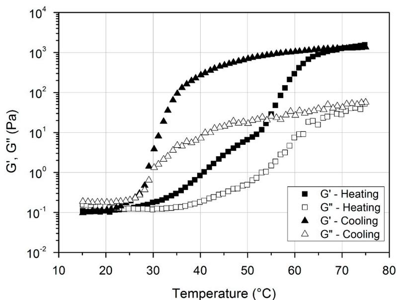
**Figure 8.** Temperature dependence of dynamic viscoelasticities for methylcellulose A4M at 10 g/L in aqueous solution. Constant frequency of 0.5 Hz, strain of 1% and temperature rate of 0.5 °C/min. ■, □ heating; ▲, Δ cooling.  $G'$  full symbols and  $G''$  open symbols. Reproduced with permission from Taylor & Francis Group, 2015 [20].
