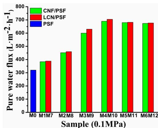
Figure 13. Pure water flux of membranes.
