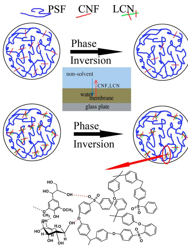
**Figure 2.** The possible membrane formation mechanism affected by the cellulose nanofibrils (CNF) and Lignocellulose nanofibrils (LCN).
