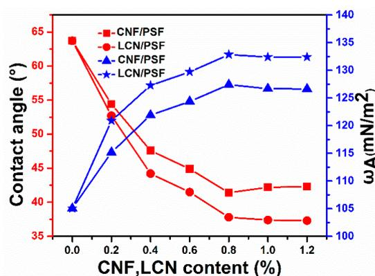
**Figure 11.** Effect of CNF and LCN contents on contact angle and surface energy of membranes.
