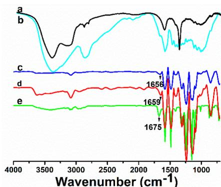
**Figure 6.** FTIR spectra of: (a) CNF; (b) LCN; (c) Sample M0 (PSF); (d) Sample M4 (CNF/PSF); and (e) Sample M10 (LCN/PSF).
