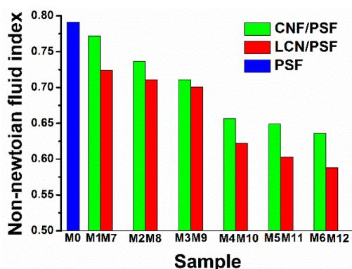
Figure 10. Non-Newtonian fluid index of membrane solutions: Sample M0–12.
