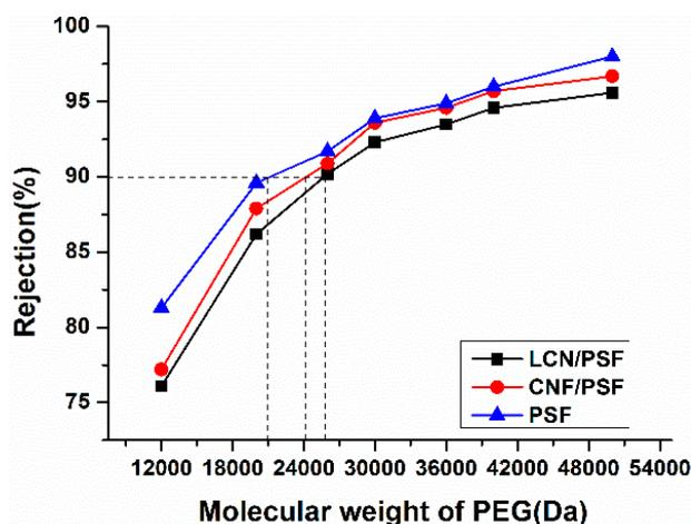
**Figure 15.** Polyethylene glycol (PEG) retention rate as a function of molecular weight for Membranes: M0, M4, and M10.
