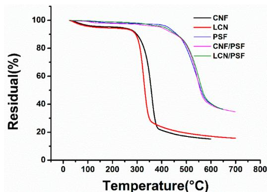
**Figure 8.** Thermal gravity analysis curves of CNF, LCN, Sample M0 (PSF), Sample M4 (CNF/PSF) and Sample M10 (LCN/PSF).
