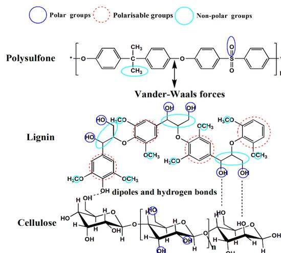
**Figure 1.** The absorption promoter mechanism of lignin on cellulose adhesion to the membrane matrix.
