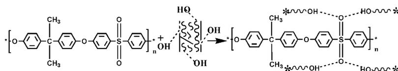
**Figure 7.** Schematic representation of the intermolecular interactions between the components in LCN/PSF ultrafiltration membranes (\* denotes LCN, ~ denotes cellulose chains, and — denotes lignin chains).
