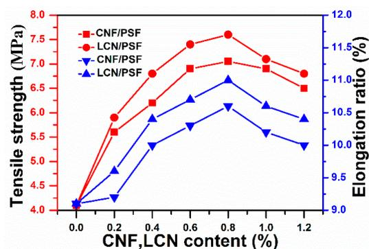
**Figure 12.** Effects of the CNF and LCN content on the tensile strength and breaking elongation of the membranes.
