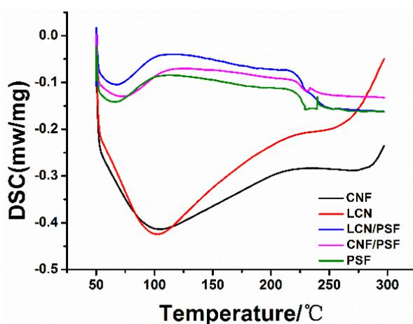
**Figure 9.** Differential scanning calorimetry curves of CNF, LCN, Sample M0 (PSF), Sample M4 (CNF/PSF) and Sample M10 (LCN/PSF).
