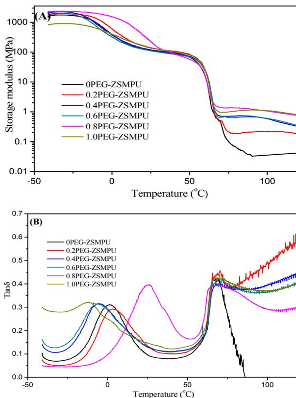
**Figure 9.** The Dynamic mechanical analysis (DMA) curves of PEG-ZSMPTUs (A) storage modulus and (B) tan δ curves.
