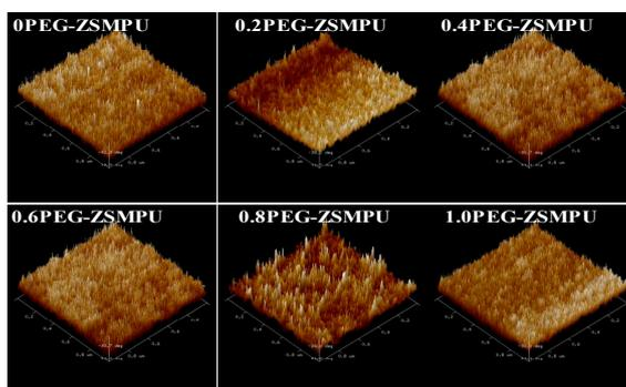
Figure 5. Atomic force microscopy (AFM) images (3D phase) of PEG-ZSMPUs.
