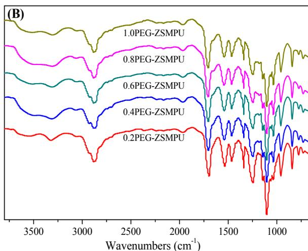
**Figure 1.** Fourier transform-infrared spectroscopy spectra (FT-IR) spectra of samples, (A) for comparisons of 1,3-PS, 0PEG-ZSMPU and 1PEG-ZSMPU; (B) for PEG-ZSMPUs with different zwitterionic hard segments.
