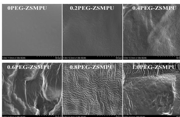
Figure 6. Scanning electron microscopy (SEM) images of PEG-ZSMPUs.
