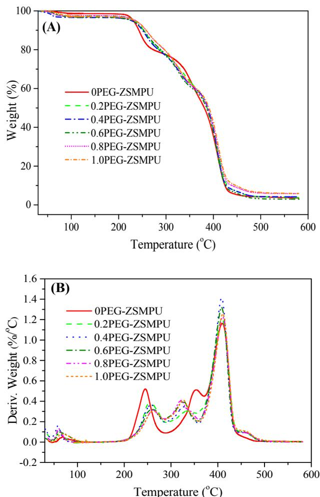
**Figure 8.** Thermogravimetric analysis (TGA curves of PEG-ZSMPUs: (A) TG curves, and (B) DTG curves).
