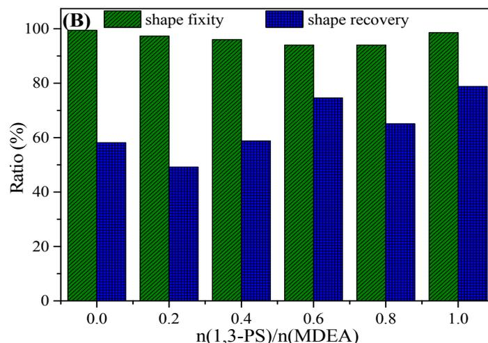
**Figure 10.** Thermal-induced shape memory effects (SMEs) of PEG-ZSMPUs: (A) shaped memory curves of sample 1.0PEG-ZSMPU and (B) shape recovery and shape fixity of PEG-ZSMPUs with various molar ratio of 1,3-PS/MDEA.
