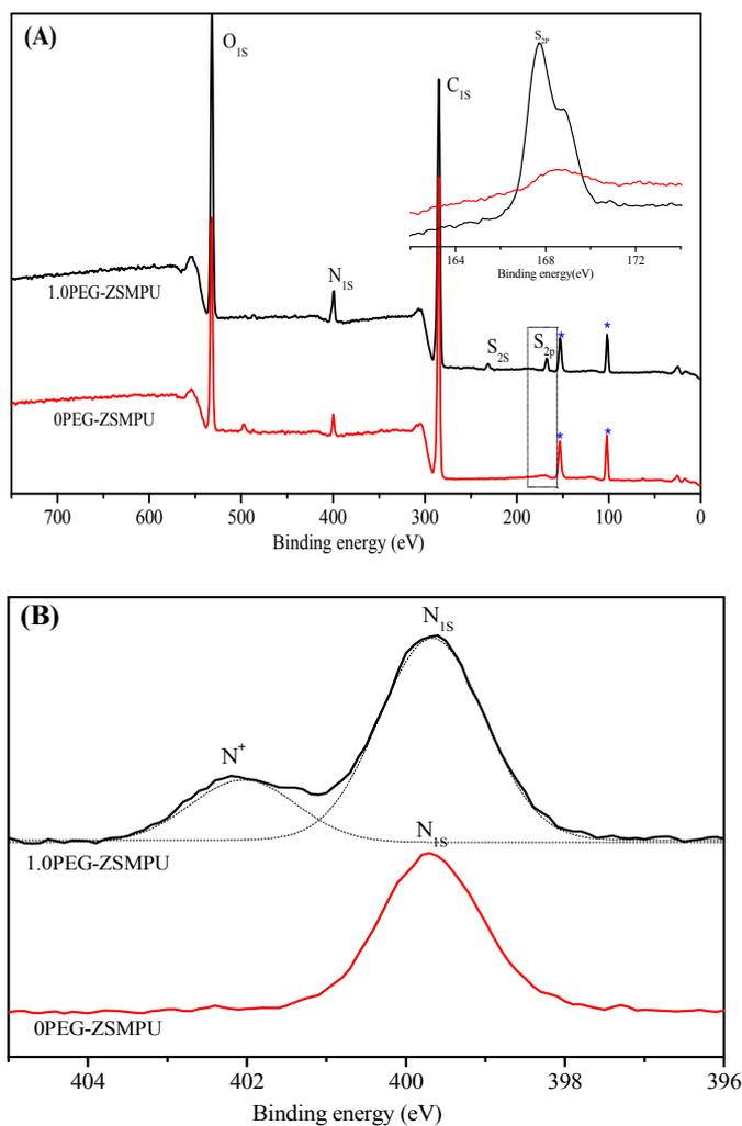
**Figure 2.** X-ray photoelectron spectroscopy (XPS) and  $N_{1s}$  spectra of 0PEG-ZSMPU and 1.0PEG-ZSMPU. ((A) Full spectra; (B)  $N_{1s}$  spectra).
