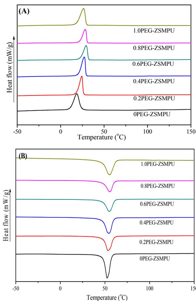
**Figure 7.** Differential scanning calorimeter (DSC) curves of PEG-ZSMPUs: (A) the cooling curves and (B) the second DSC heating curves.
