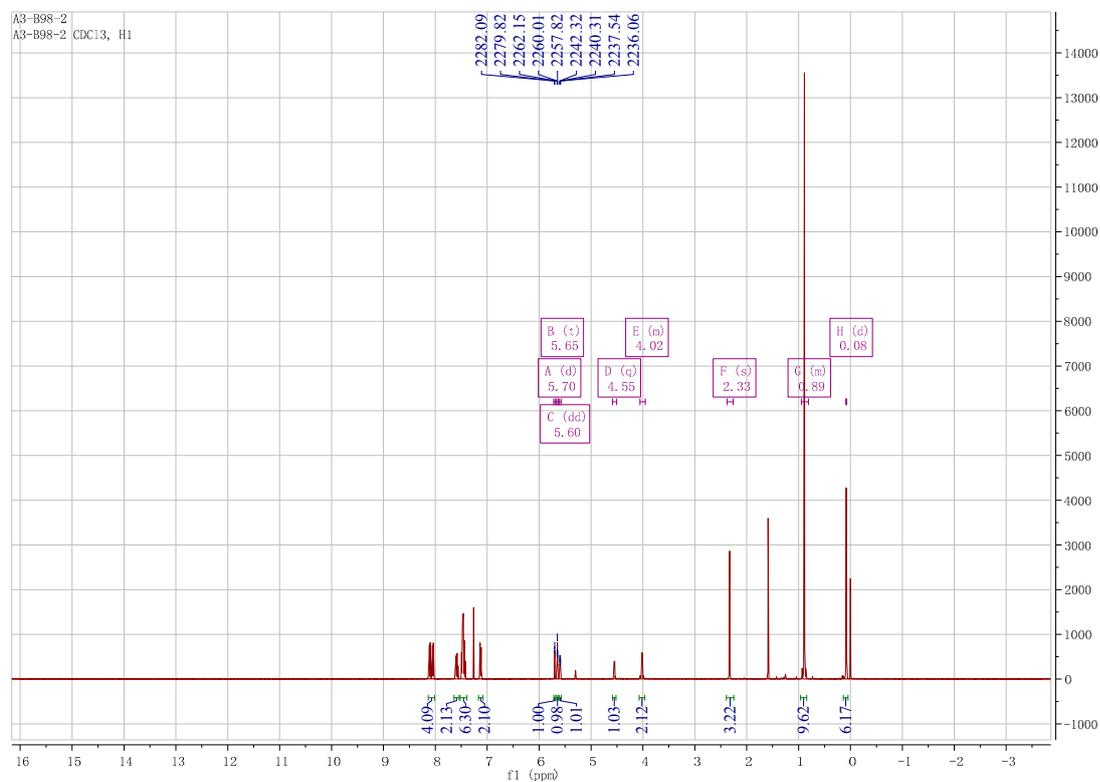
Figure S18. <sup>1</sup>H-NMR (CDCl<sub>3</sub>, 400 MHz) of 4
