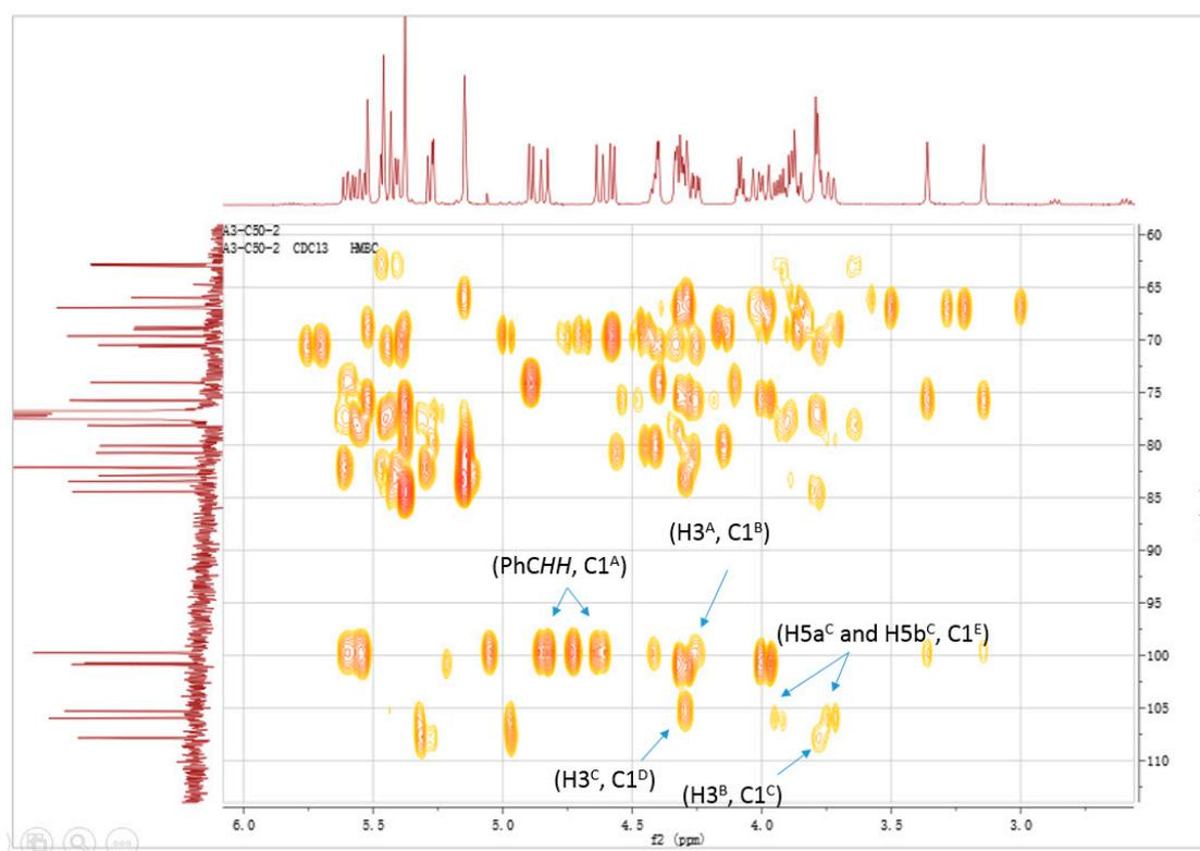
**Figure S42.**  $^1\text{H}$ - $^{13}\text{C}$  HMBC (CDCl<sub>3</sub>, 125 MHz) of 17
