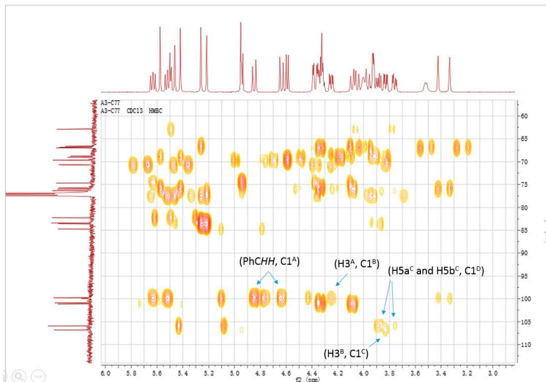
Figure S52.  $^1\text{H}$ - $^{13}\text{C}$  HMBC ( $\text{CDCl}_3$ , 125 MHz) of 20
