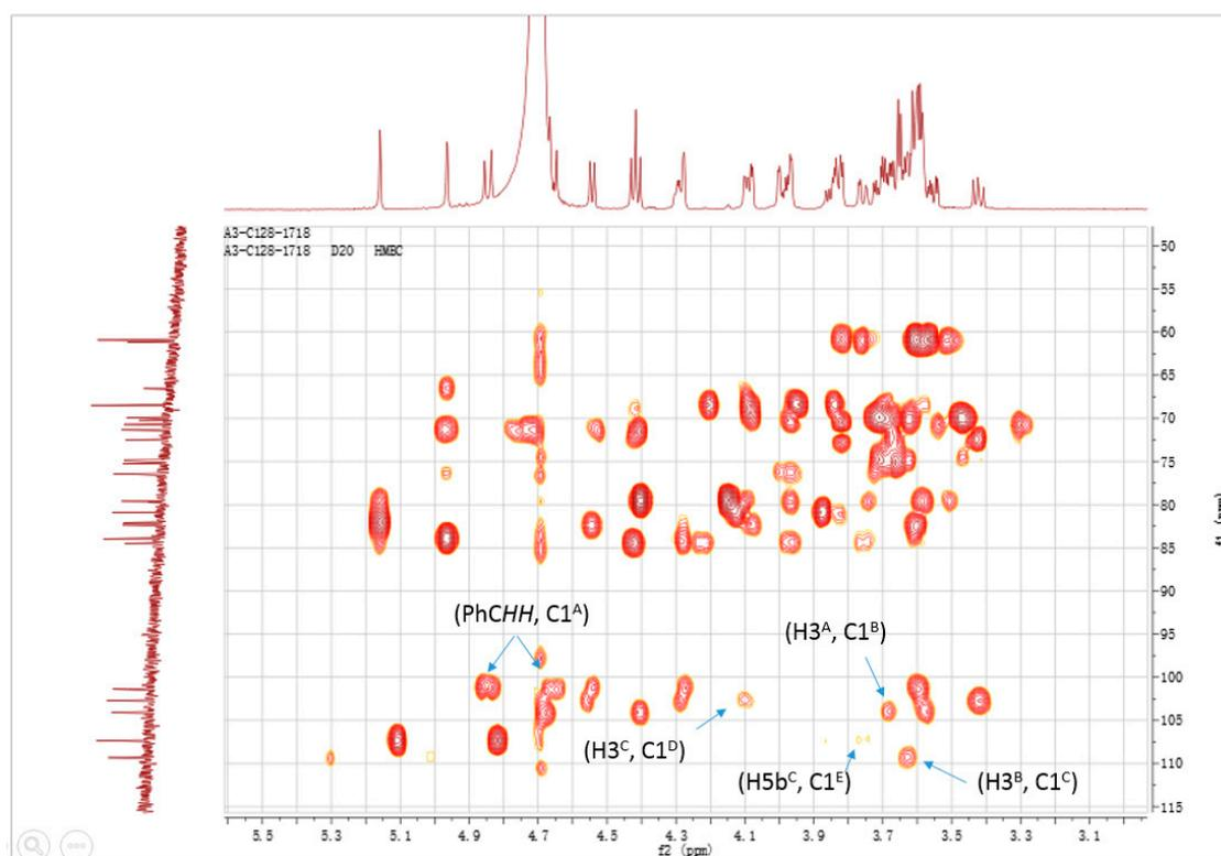
Figure S74.  $^1\text{H}$ - $^{13}\text{C}$  HMBC (CDCl<sub>3</sub>, 125 MHz) of 27
