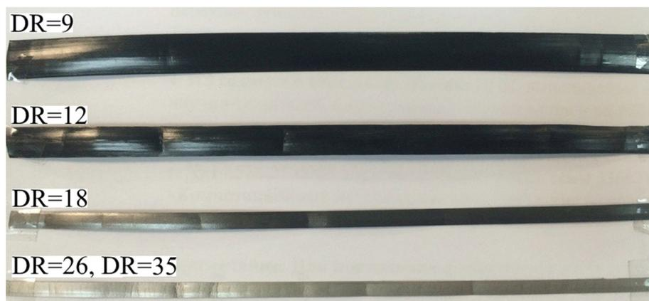
**Figure 3.** Photo of bulk oriented films based on UHMWPE/1% FMWCNT with different draw ratios (DR). DR is indicated in the figure.
