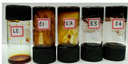
**Figure 2.** Prepared liquid electrolyte (LE) and electrolytes containing 1, 1.2, 1.4, and 1.6 starch (E1, E2, E3, and E4 respectively).
