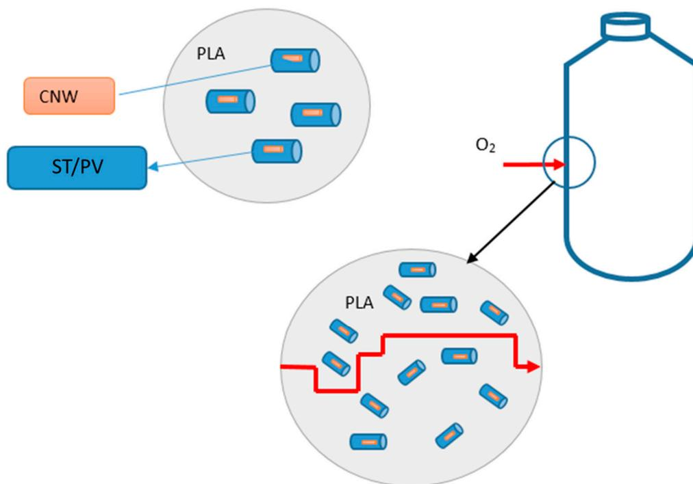
**Figure S1.** Schematic representation of the tortuous diffusion path generated by CNC containing fibers (PVST/CNC) into PLA materials.
