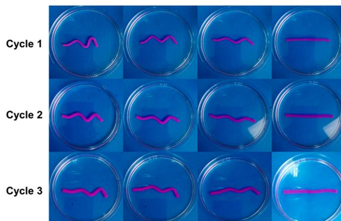
**Figure S8.** Cycled multiple shape memory behavior of the PAAm-CS hydrogel via CS physical microcrystal crosslink interaction. NaOH solution (75 mM) and HCl (100 mM) were used for shape memory and shape recovery procedures, respectively.
