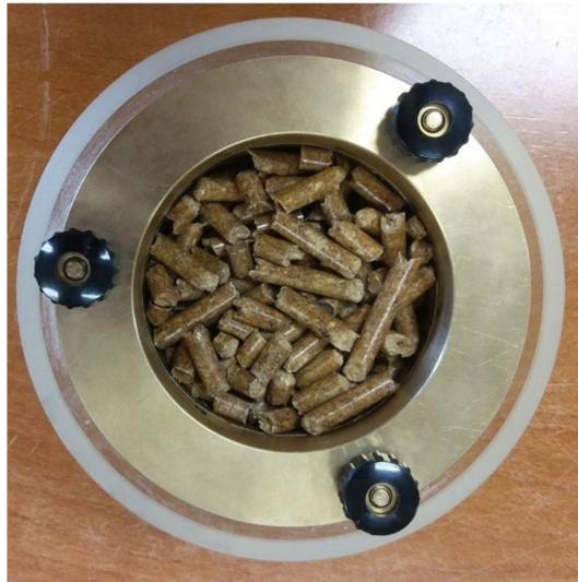
**Figure 5.** A sample of wood pellets inside one of the oedometric cells.
