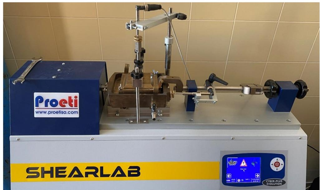
**Figure 2.** Semi-automatic direct shear test device.
