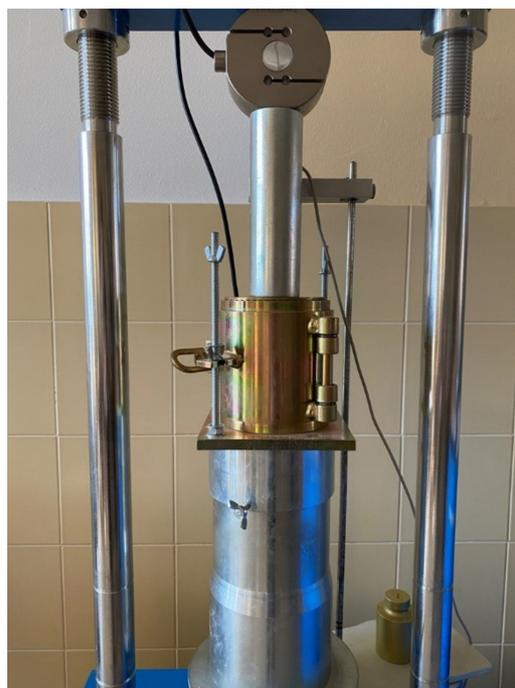
**Figure 6.** Normal Proctor mould in the multiuse press, used to determine the apparent specific weight of the test materials under normal stress.
