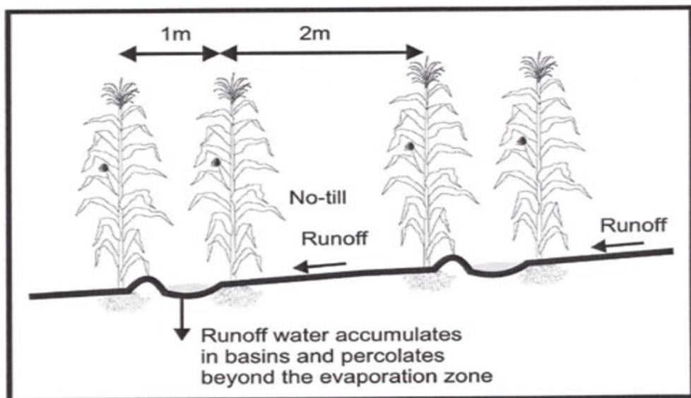
**Figure 1.** Schematic diagram of the in-field rainwater harvesting technique (after Hensley et al. [8]).
