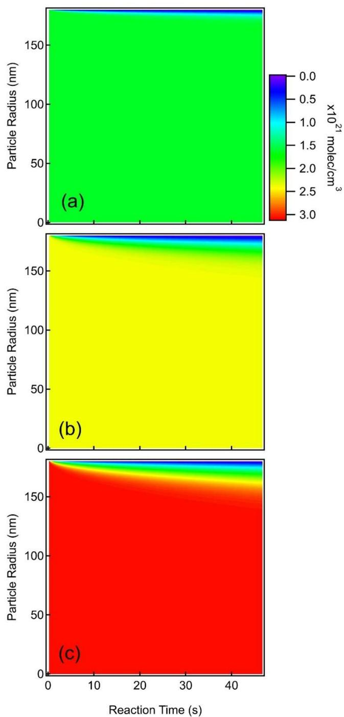
**Figure S8.** Modeled space-time plots of MGP concentration for MGP:lactose molar ratios of (a) 1:1 (b) 2:1 and (c) 4:1 with a constant OH gas number density of  $1.08 \times 10^{10}$  cm<sup>-3</sup>. The particle radius is 180 nm and the reaction time is 46 s.
