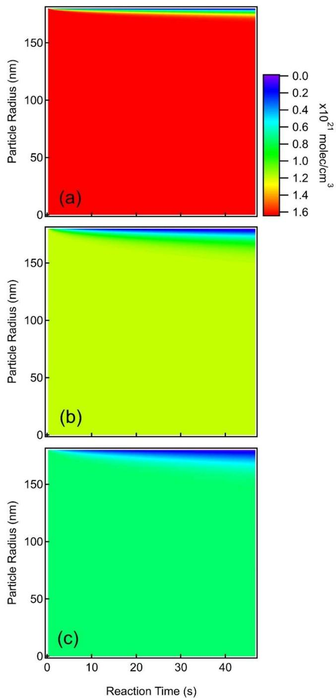
**Figure S7.** Modeled space-time plots of lactose concentration for MGP:lactose molar ratios of (a) 1:1 (b) 2:1 and (c) 4:1 with a constant OH gas number density of  $1.08 \times 10^{10}$  cm<sup>-3</sup>. The particle radius is 180 nm and the reaction time is 46 s.
