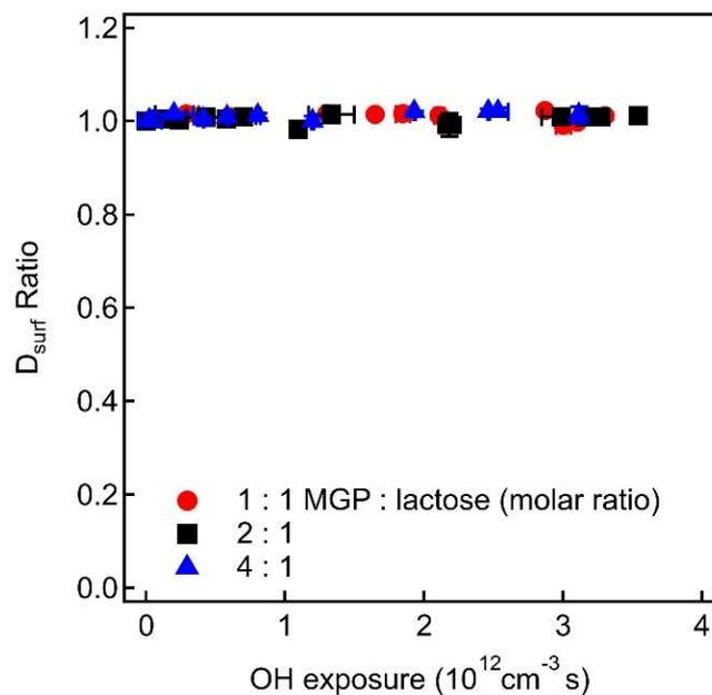
**Figure S5.** Relative surface weighted diameter as a function of OH exposure for MGP:lactose molar ratios of 1:1 (red solid circles), 2:1 (black solid squares), 4:1 (blue solid triangles) used for the GC-MS experiments at WVU. The error bar is  $2\sigma$  of the mean values.
