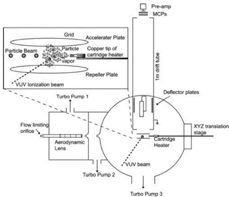
**Figure S2.** Schematic view of the aerosol TOF-MS at the Advanced Light Source synchrotron. The sampling of the particle flow is performed using an aerodynamic lens system generating a collimated particle beam under vacuum. The particles are vaporized by a cartridge heater in the ionization region (see insert) and the resulting plume is ionized by the VUV light. The ions are mass selected by a linear time-of-flight mass spectrometer. Reproduced from Mysak et al. (2005) [48].
