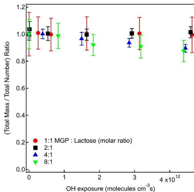
**Figure S4.** Ratio of the reacted over unreacted aerosol total mass as a function of OH for MGP:lactose molar ratios of 1:1 (red solid circles), 2:1 (black solid squares), 4:1 (blue solid up-triangles), and 8:1 (green solid down-triangles) used for the VUV-AMS experiments at the ALS. The error bar is  $2\sigma$  of the mean values.
