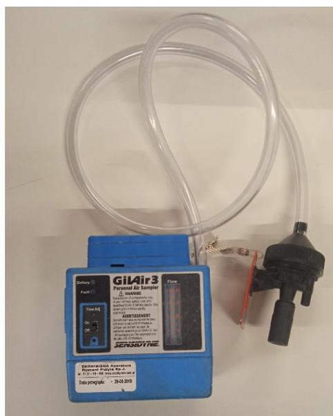
**Figure 2.** The sampling apparatus applied for dynamic sampling. It includes the air sampling pump and cyclone head for collection of the respirable fraction of dust. Samples collected on quartz filters were analyzed for EC using TOA.
