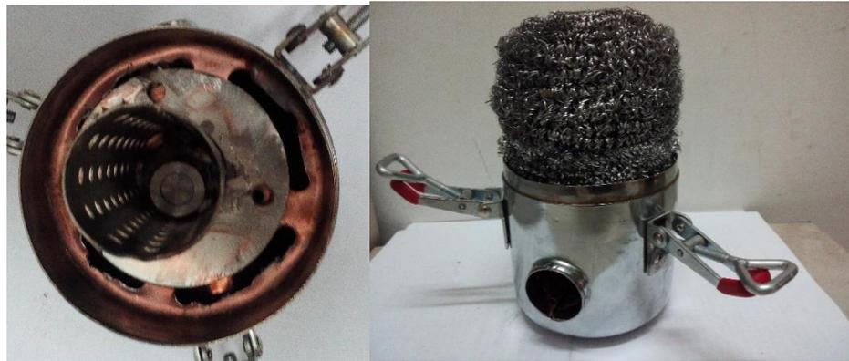
**Figure 13.** Inside view of the optimized muffler; the muffler filled with stainless steel fibers.
