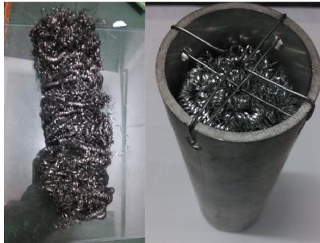
**Figure 3.** Stainless steel fiber particulate filter setup to verify the filtration performance.
