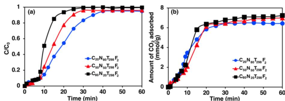
**Figure 2.** Effect of CO<sub>2</sub> composition on CO<sub>2</sub> adsorption at 298 K and feed flow rate of 2 L/h, which listed as: (a) breakthrough curves; (b) adsorption capacity.
