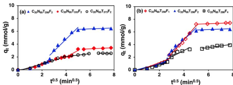
Figure 7. Intraparticle diffusion model plots of CO<sub>2</sub> adsorption on zeolite 5A at (a) different temperatures; (b) different feed flow rates.
