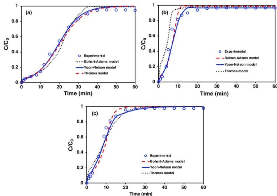
**Figure 5.** CO<sub>2</sub> adsorption on zeolite 5A results with different breakthrough curve models under different operating conditions of: (a) 298 K with 2 L/h feed flow rate; (b) 373 K with 2 L/h feed flow rate; (c) 298 K with 4 L/h feed flow rate.
