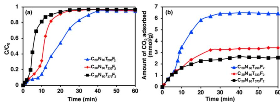
**Figure 3.** Effect of temperature on CO<sub>2</sub> adsorption at feed flow rate of 2 L/h, which represented as: (a) breakthrough curves; (b) adsorption capacity.
