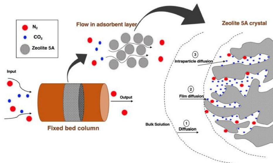
**Figure 9.** Adsorption mechanisms of CO<sub>2</sub> adsorption from CO<sub>2</sub>/N<sub>2</sub> gas mixture on zeolite 5A.
