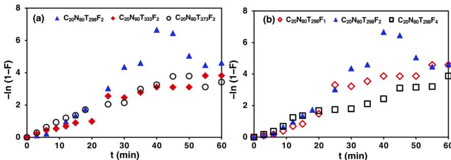
Figure 8. Boyd model plots of CO<sub>2</sub> adsorption on zeolite 5A at (a) different temperatures; (b) different feed flow rates.
