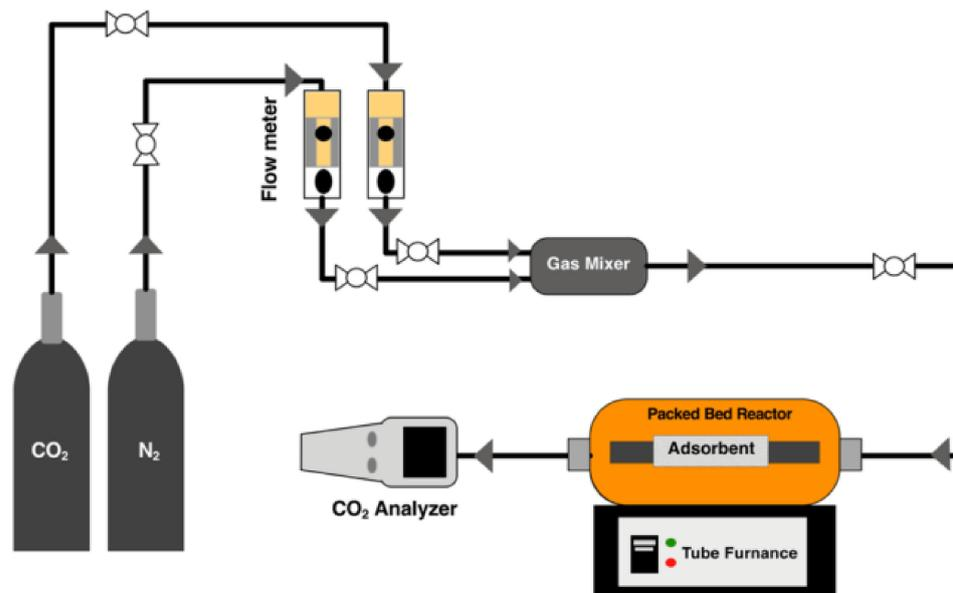
**Figure 1.** Process of CO<sub>2</sub> adsorption from CO<sub>2</sub>/N<sub>2</sub> gas mixture with fixed-bed reactor.
