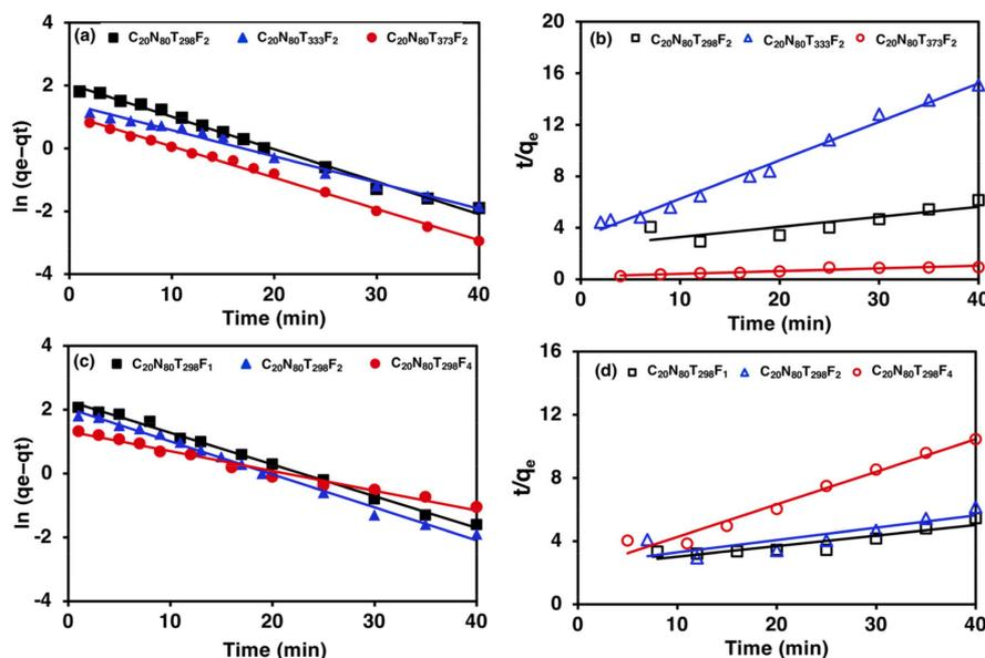
**Figure 6.** Kinetic parameters models of CO<sub>2</sub> adsorption using zeolite 5A: (a) PFO model at different temperatures; (b) PSO model at different temperatures; (c) PFO model at different feed flow rates; (d) PSO model at different feed flow rates.
