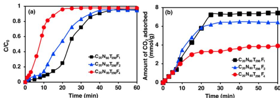
**Figure 4.** Effect of feed flow rate on CO<sub>2</sub> adsorption at 298 K, represented as: (a) breakthrough curves; (b) adsorption capacity.
