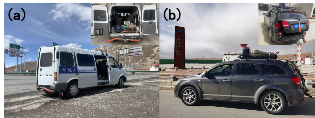
Figure 2. Vehicle PEMS testing schematic. (a) China IV diesel vehicle, (b) China V gasoline vehicle.
