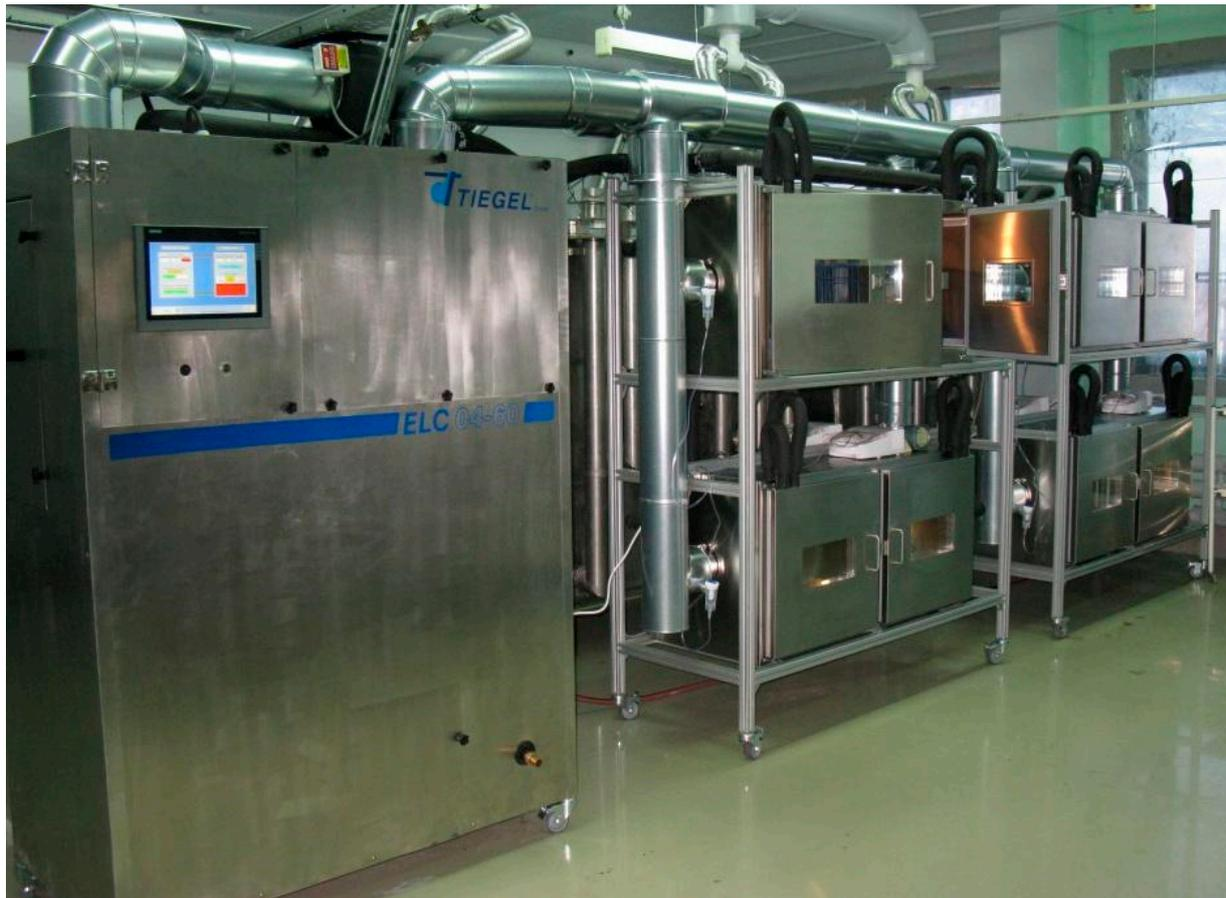
**Figure 1.** TIEGEL ELC 04-60 dynamic aerobiology chamber.
