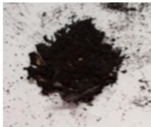
**Figure 2.** An example of chimney deposit (soot) sample collected from the inner surface of the chimney. In order to obtain access to the deposit, the second part of the chimney device was separated from the whole chimney system, and then soot samples were collected at selected heights using a spoon for the lower levels and an elongated brush tool for the higher levels.
