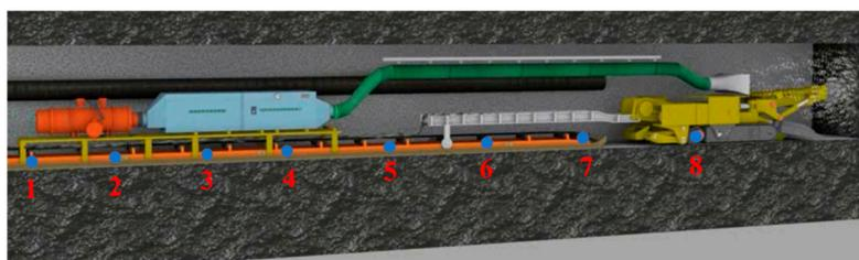
**Figure 3.** Layout of monitoring points in the underground roadway.
