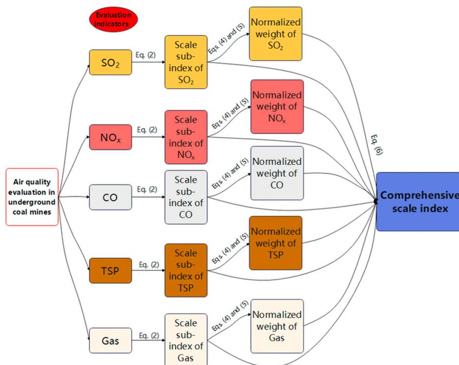
**Figure 2.** Frame diagram of generalized contrastive weighted comprehensive scale index evaluation model.
