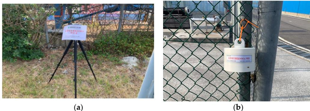
**Figure 2.** VOC Capture Methods: (a) Active Sampling (b) Passive Sampling. The meaning of the phrase in the figure is ‘Measuring VOCs’.
