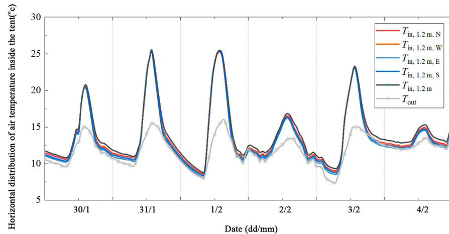
**Figure 7.** Horizontal distribution of air temperature in a tent under unregulated winter conditions.
