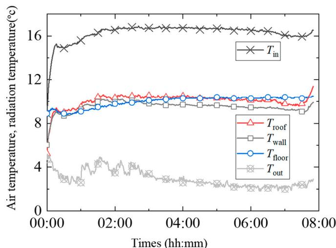
**Figure 18.** The inner surface temperature and air temperature of the tent under heating conditions in winter.
