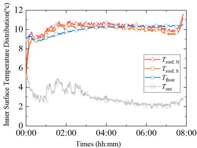
Figure 17. Tent top surface temperature and ground temperature under winter heating conditions.
