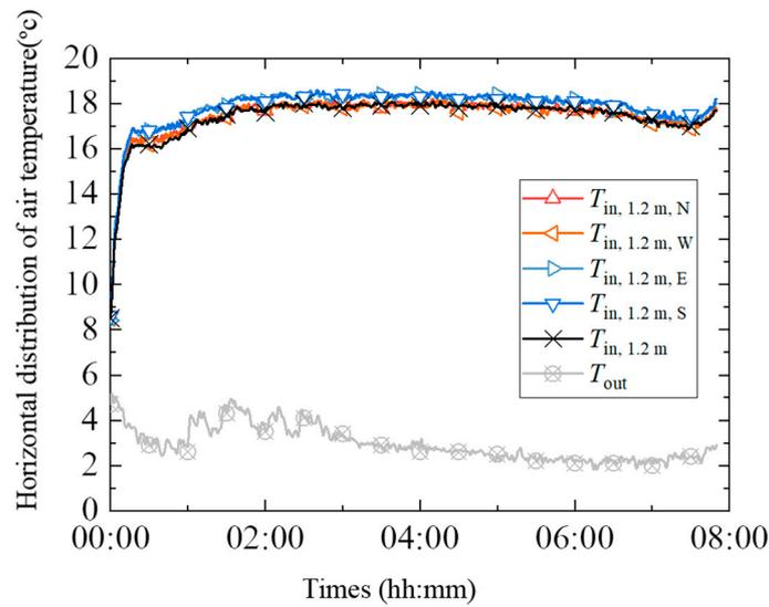
**Figure 14.** Horizontal distribution of air temperature in the tent under winter heating conditions.
