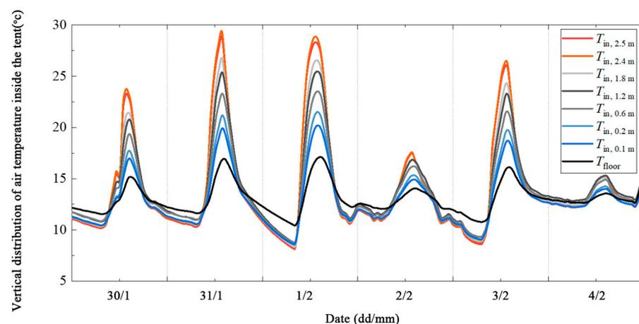
**Figure 8.** Vertical distribution of air temperature in a tent under unregulated winter conditions.
