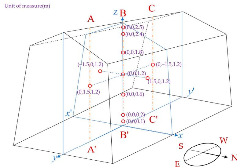
A, B, C and A', B', C' play a role in dividing the space inside the tent, helping to visually and objectively determine the specific location of the temperature sensor.
