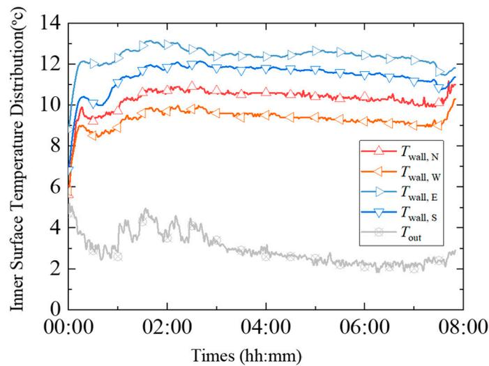
Figure 16. The internal surface temperature around the tent under winter heating conditions.
