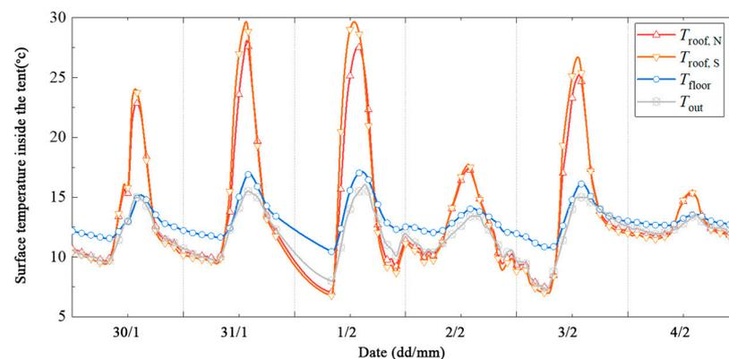
**Figure 10.** The top surface temperature and ground temperature inside the tent under unregulated winter conditions.
