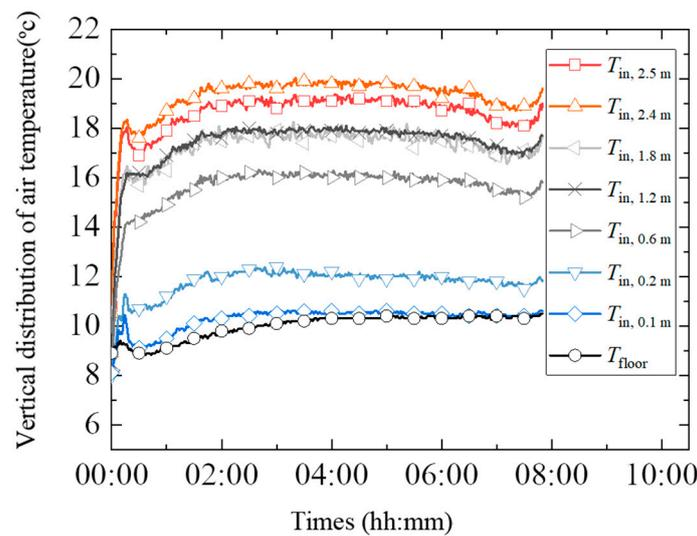
**Figure 15.** Vertical distribution of air temperature in the tent under winter heating conditions.
