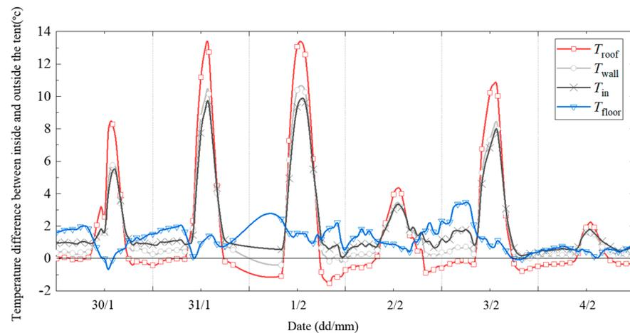
**Figure 12.** The difference between the temperature inside the tent and the ambient temperature under unregulated winter conditions.
