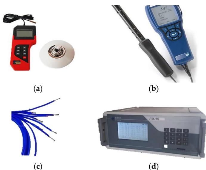
**Figure 5.** Experimental testing instruments: (a) solar radiation recorder; (b) indoor air quality tester; (c) point thermocouple sensor; (d) multichannel automatic temperature and heat flow recorder.
