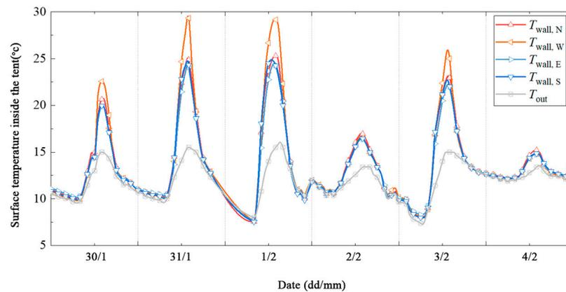
**Figure 9.** The inner surface temperature around the tent under unregulated winter conditions.
