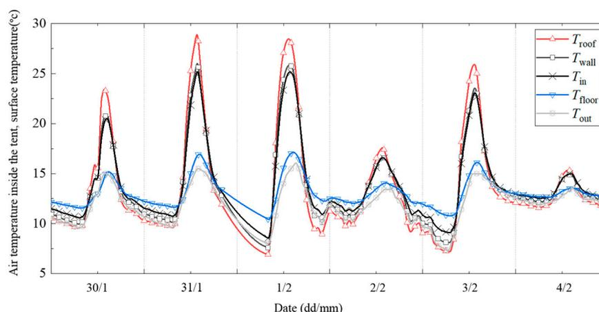
**Figure 11.** The inner surface temperature and air temperature of the tent under unregulated winter conditions.
