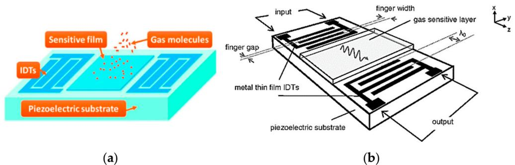
Figure 13. Overview of AGS [66,67]. (a) Architecture. (b) Working principle.
