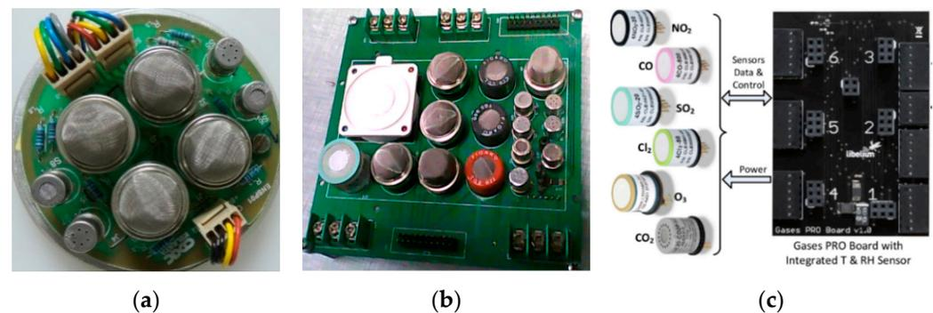
**Figure 17.** Major contributions in applied GSAs, GSGs, and ENBs. (a) Test GSG for I-AQA [70]. (b) Eighteen-parameter GSA [71]. (c) Smart rig test ENB [72].
