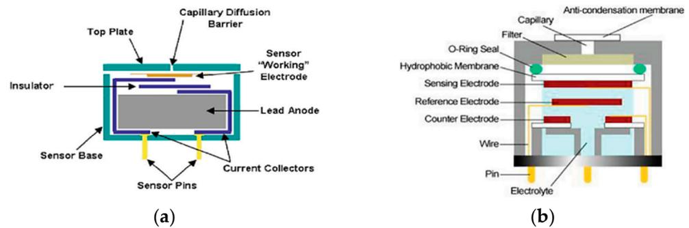
**Figure 10.** Overview of ECS [56–58] (a) Architecture. (b) Working principle.
