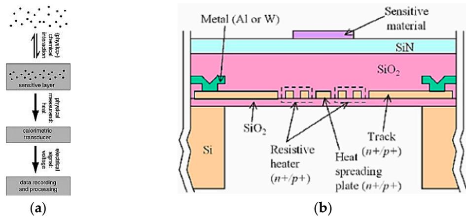
Figure 12. Overview of CMGS [63–65]. (a) Architecture. (b) Working principle.
