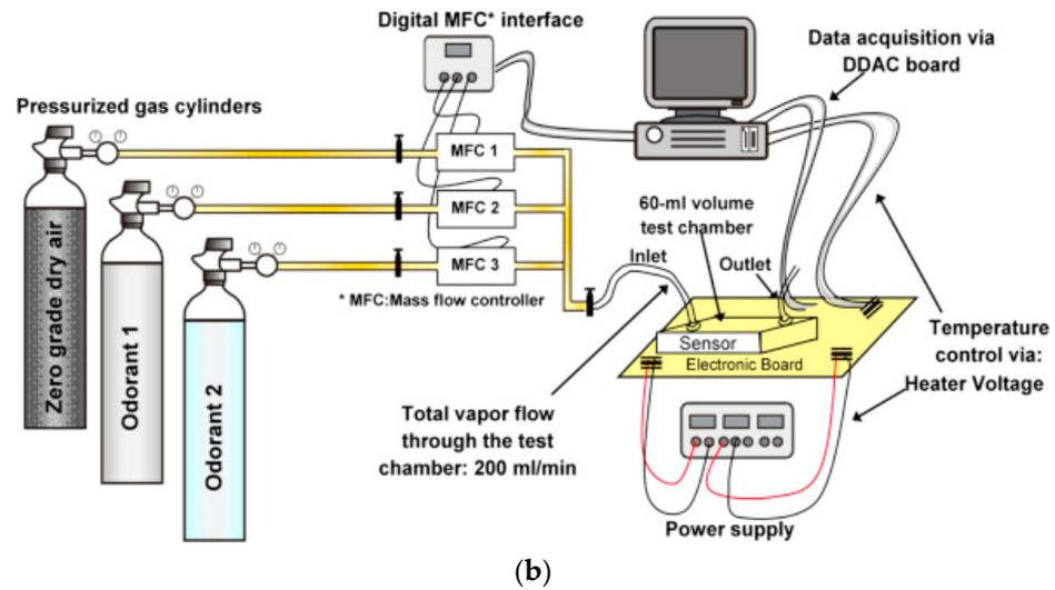
Figure 20. The computer-supervised AQGS testing systems [80,81]. (a) AQGS array testing and calibration system [80]. (b) The ENB testing and calibration system [81].
