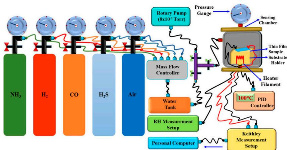
Figure 22. Air quality mesh network testing and calibration system [92].
