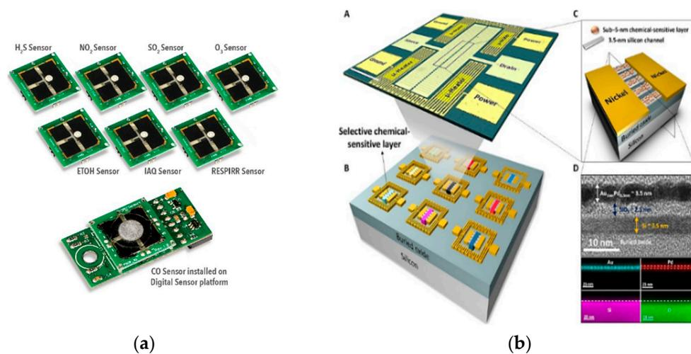
**Figure 18.** Major contributions in GSAoC-based SOI for applied GSGs and ENBs. (a) SPEC DSPoC with GSA on chip [73–76]. (b) Monolithic GSA on chip with 3.5 nm wires [77].
