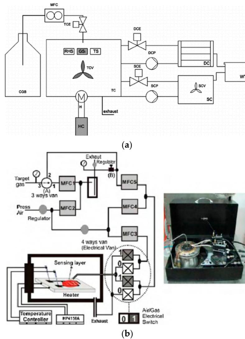
**Figure 19.** The AQ gas sensor calibration chamber-based system [74]. (a) P&ID of a unit AQGS testing and calibration system. (b) System assembly and architecture.
