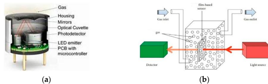
**Figure 8.** Overview of OGS [50,53]. (a) Architecture. (b) Working principle.
