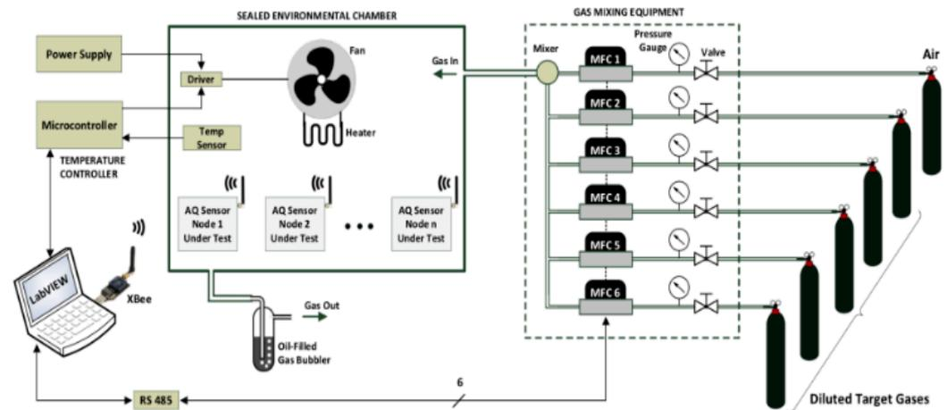
Figure 21. IoT-based Smart AQ GSA testing and calibration system [84].
