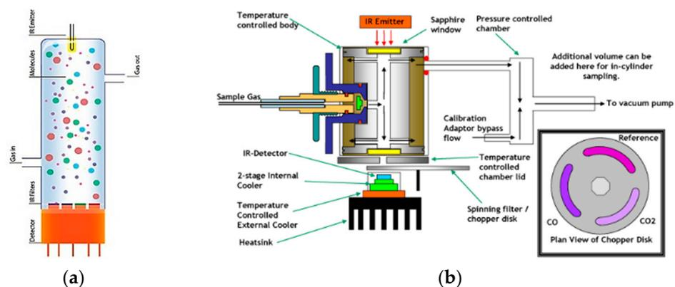
**Figure 9.** Overview of NDIR-GS [55,56] (a) Architecture. (b) Working principle.
