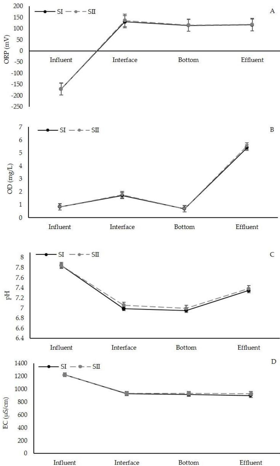
**Figure 6.** Internal conditions of the PS VF wetlands during the study: Oxidation-reduction potential (ORP) (A), OD (B), pH (C), electric conductivity (EC) (D).
