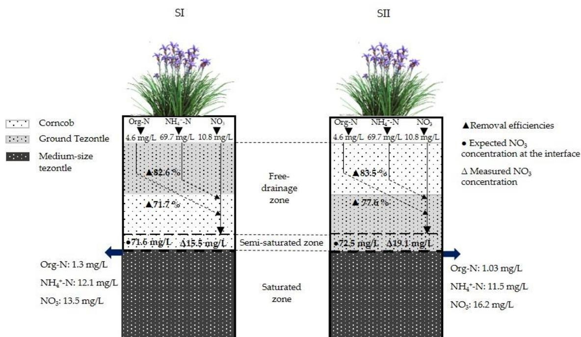
Figure 13. Theoretical generation of nitrate: Difference between expected concentrations through full nitrification and measured concentrations.
