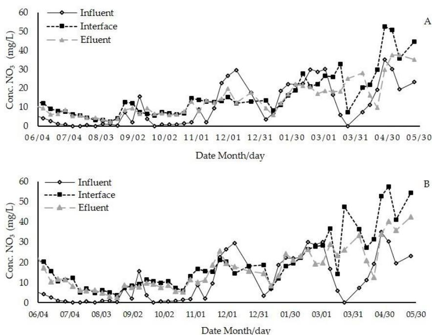
**Figure 11.** Measurements of nitrate at three points in system I (SI) (A) and system II (SII) (B) during the study.
