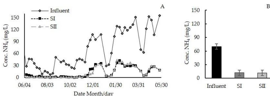
**Figure 9.** Ammonium concentrations in the study with PS VF wetlands, (A) values along the sampling campaigns, (B) mean concentrations ( $\pm$  standard error) throughout the period of study.
