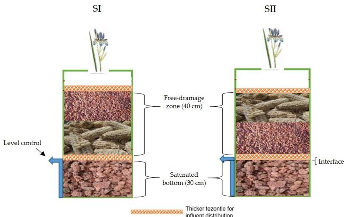
**Figure 1.** Two pilot-scale partially saturated (PS) vertical flow (VF) wetlands for nitrogen removal.
