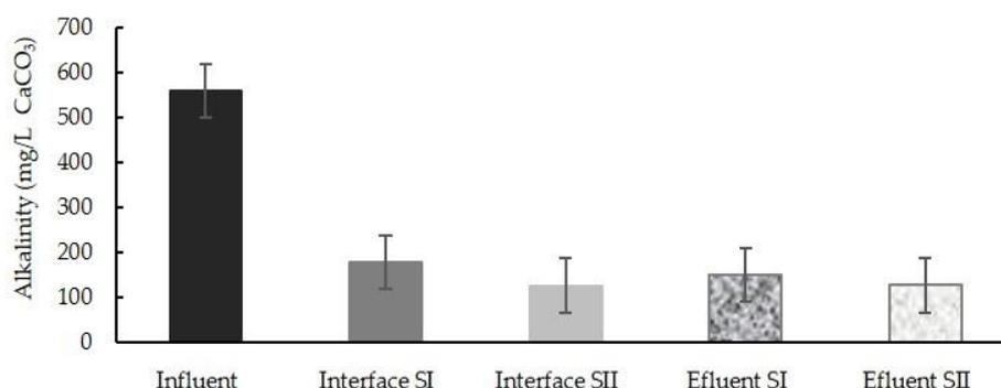
Figure 7. Alkalinity measurements in the two PS VF wetlands.
