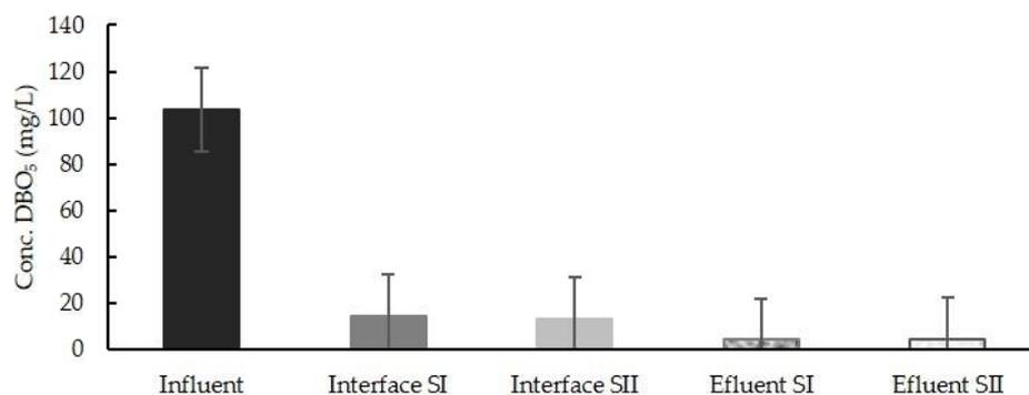
**Figure 3.** Comparison of BOD<sub>5</sub> concentrations at the three points of the PS VF wetlands during the last 23 weeks of the study.
