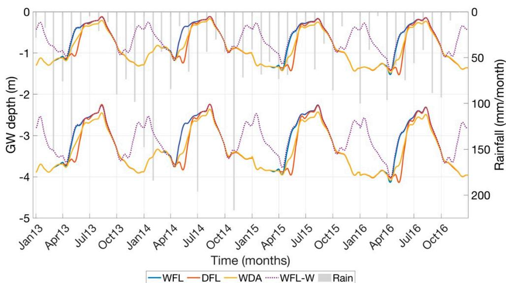
**Figure 12.** Simulated groundwater levels (both for shallow and deep GW zones) during the agricultural season 2013–2016 for the four irrigation scenarios.
