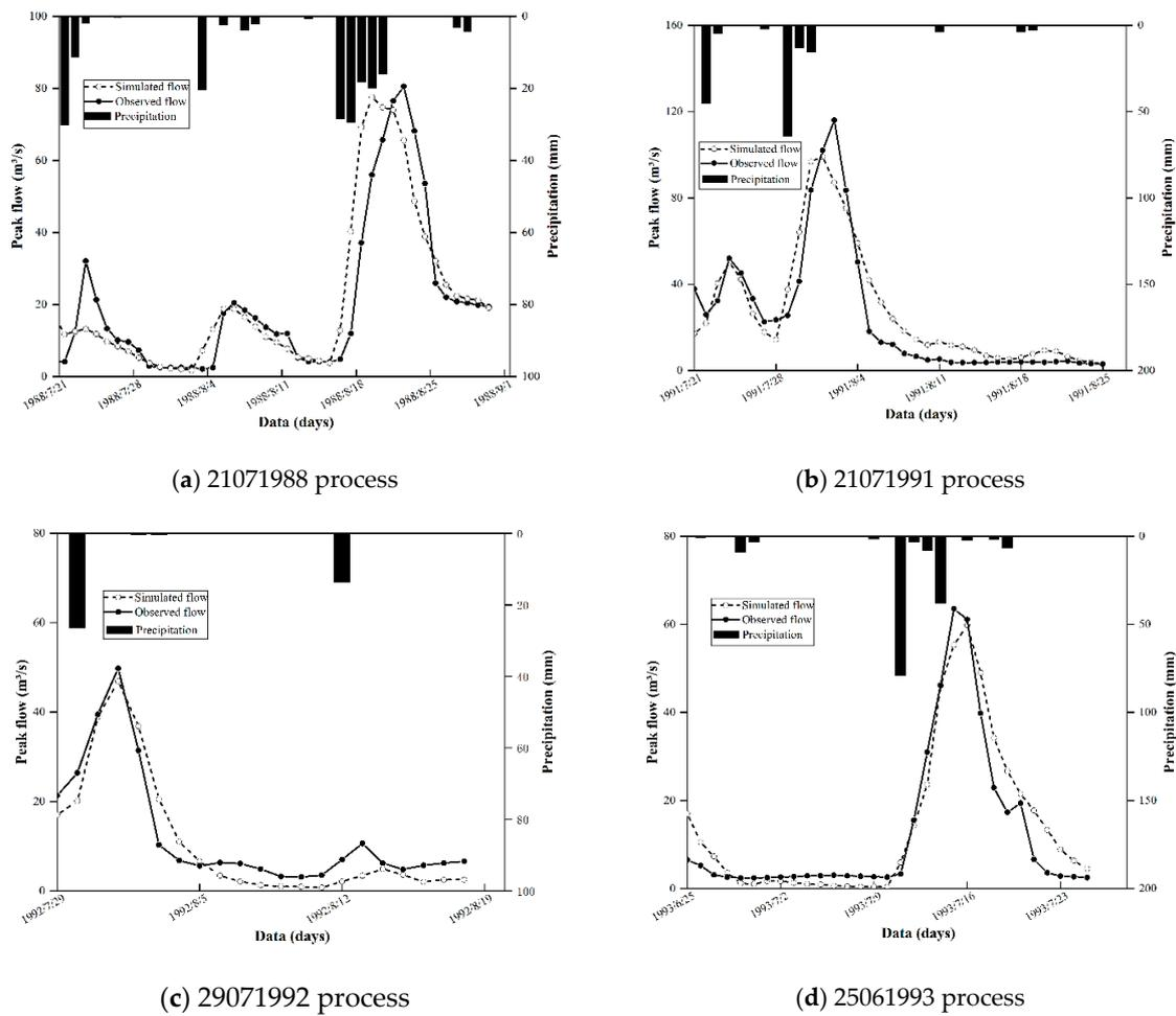
Figure 4. Comparison between simulation and observation in validation period before urbanization.
