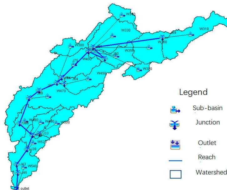
**Figure 2.** HEC-HMS conceptual model for Pu River Basin.**Table 3.** Characteristic values of each sub-basin in the study area.
