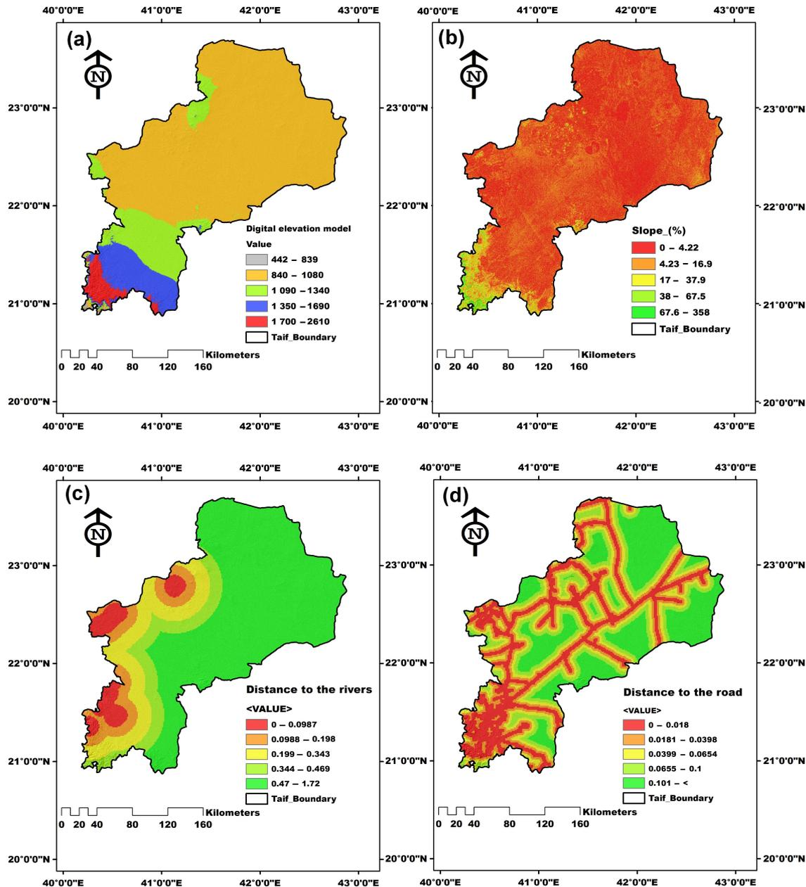
Figure 2. A multi-layered perspective: mapping DEM (a), slope (b), road distance (c), and river distance (d).
