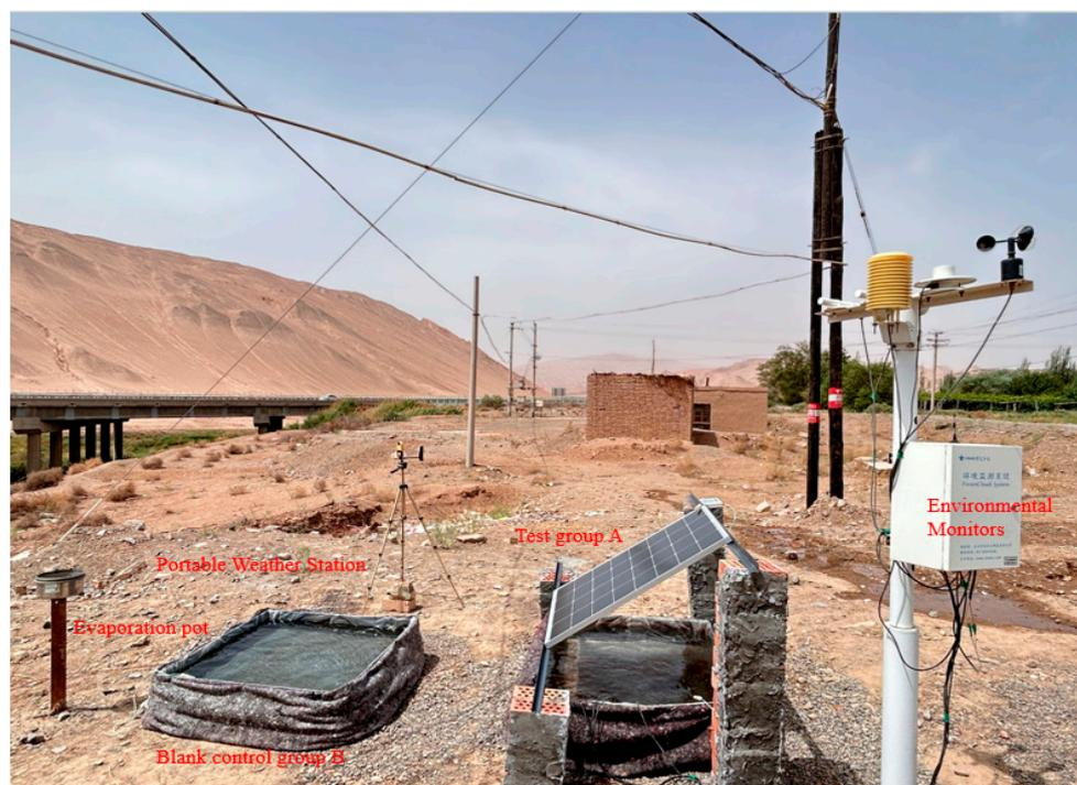
**Figure 4.** Water-based piled PV test diagram.
