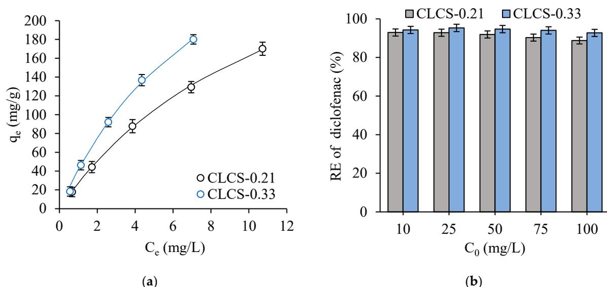
**Figure 2.** Adsorption isotherms of diclofenac on CLCS-0.21 and CLCS-0.33 (a) at 20 °C temperature (symbols represent experimental data and lines show the fitted curves of the Langmuir adsorption model) and the amount of removed diclofenac depending on the initial concentration of diclofenac in water (b). Concentrations of adsorbate solutions: 10, 25, 50, 75, and 100 mg/L.
