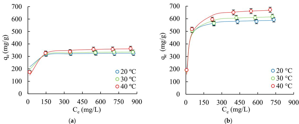
**Figure 1.** Adsorption isotherms of diclofenac on CLCS-0.21 (a) and CLCS-0.33 (b) at different temperatures. Symbols represent experimental data and lines show the fitted curves of the Langmuir adsorption model. Concentrations of adsorbate solutions: 100, 300, 500, 700, 850, and 1000 mg/L.
