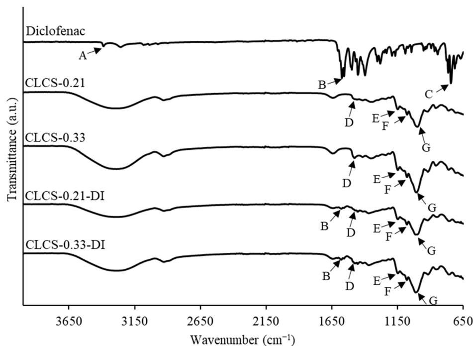
**Figure 5.** FT-IR spectra of diclofenac, CLCS-0.21, CLCS-0.33, CLCS-0.21-DI, and CLCS-0.33-DI. The letters indicate the peaks at respective wavenumber: A— $3387\text{ cm}^{-1}$ , B— $1576\text{ cm}^{-1}$ , C— $745\text{ cm}^{-1}$ , D— $1477\text{ cm}^{-1}$ , E— $1145\text{ cm}^{-1}$ , F— $1073\text{ cm}^{-1}$ , G— $1000\text{ cm}^{-1}$ .
