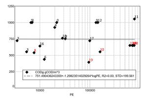
**Figure 14.** Resulting *COD* concentrations in the wastewater. (A linear regression line is plotted as grey dotted line which appears as solid grey line in the plots).
