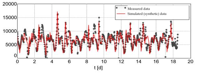
Figure 17. Synthetic inflow data (NH<sub>4</sub>-N load in kg/d) compared with measured data.
