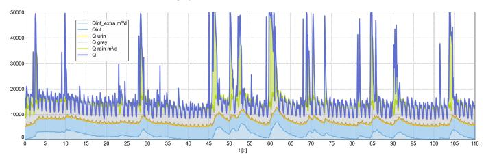
**Figure 7.** Inlet divided into additional infiltration water, infiltration water, urine, grey water, and rainwater runoff.
