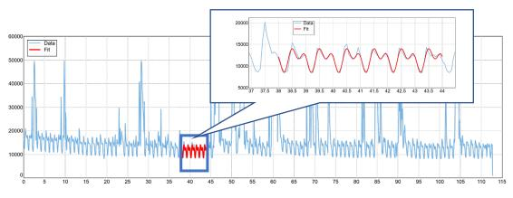
Figure 6. Inlet flow data with dry weather period.
