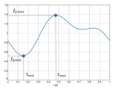
Figure 2. Fourier approximation of the dry weather inflow Langergraber et al. 2008 [5].
