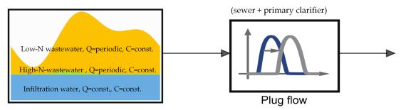
Figure 1. Modelling approach for dry weather inflow Langergraber et al. 2008 [5].
