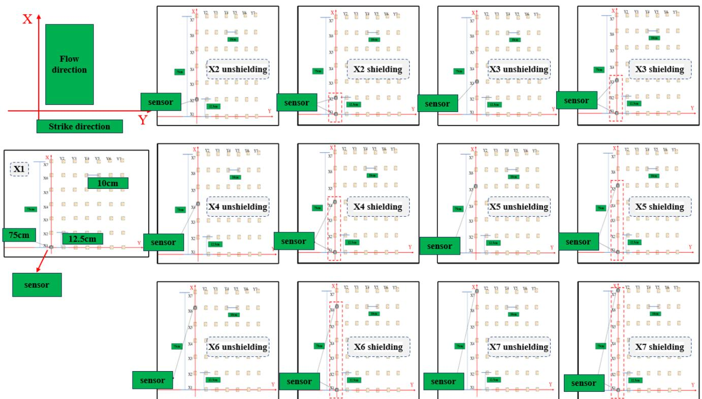
Figure 6. Arrangement of different flow directions of sensors.
