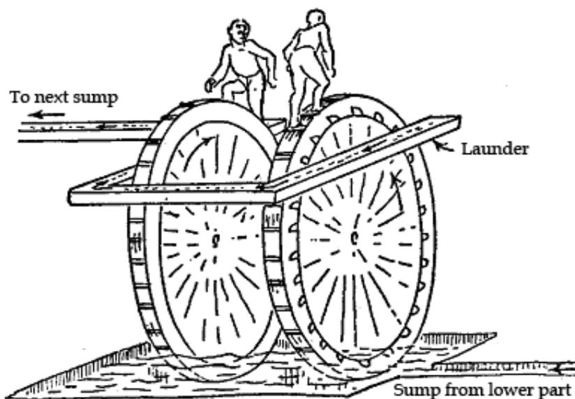
**Figure 4.** Waterwheels with *compartments rim*; representation based on archeological findings in Spain (adapted from [28]).
