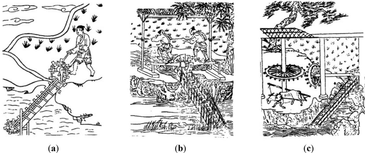
**Figure 15.** Three types of *Dragon backbones* during the Tang and Song dynasties: (a) hand-operated; (b) foot operated; and (c) oxen powered [40].
