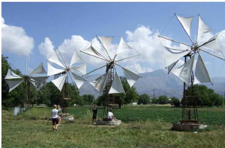
**Figure 17.** Water pumping sail-wing machines in the plateau of Lassithi in the Island of Crete (adapted from [64]).
