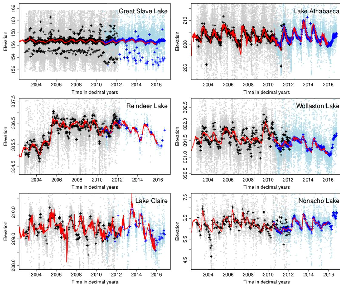
**Figure 6.** Water level time series for the six Canadian lakes: Great Slave, Athabasca, Wollaston, Claire, Nonacho, and Reindeer. The gray (Envisat) and blue (CryoSat-2) circles represent the raw retracked water levels. The black (Envisat) and blue (CryoSat-2) crosses represent the predicted water level, and the red line is the in situ water levels.
