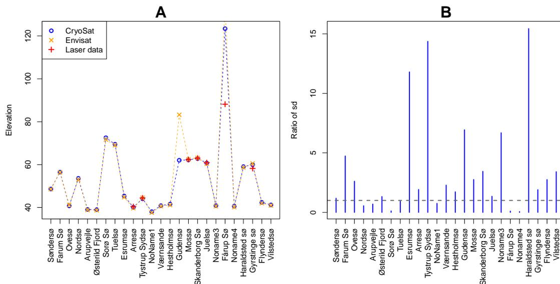
**Figure 7.** (A) the WGS84 elevations for the Danish lakes based on laser scanner data, CryoSat-2 and Envisat; (B) the ratio [Envisat/CryoSat-2] of the standard deviation of the estimated mean water level.
