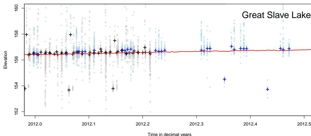
**Figure 8.** The water level time series of Great Slave Lake between January 2012 and May 2012. The gray (Envisat) and blue (CryoSat-2) circles represent the raw retracked water levels. The black (Envisat) and blue (CryoSat-2) crosses represent the predicted water level, and the red line is the in situ water levels.
